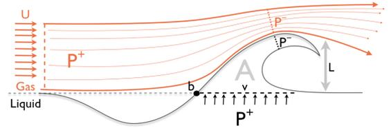
FIG. 3: Schematic representation of the wave as an obstacle to the gas stream. The acceleration of the gas stream above the wave induces a pressure drop. The pressure gradient  $(P^+ - P^-)/L$  sucks liquid into the wave.
