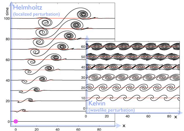
FIG. 1: Kelvin-Helmholtz instability excited by two types of initial perturbation, shown by the deformation of the interface.  $We = 1000$ ,  $Re = 100$ . The two fluids have the same density ( $r = 1$ ). For the wavelike initial condition, we observe the familiar roll-up of the interface in vortices whose size is fixed by the initially imposed wavelength. For the localized initial perturbation, we observe the creation of a system of two vortices growing in size without alteration in shape.
