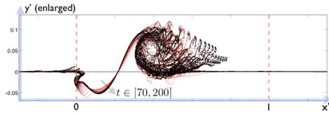
FIG. 5: Wave interface overlapped in time, recast in the self-similar reference frame  $(x', y')$  for density ratio  $r = 0.1$ . We can observe the self-similar shape of the wave, disturbed by instationarity at the wave tip and drop shedding. We see on figure 4 that the initial transient for  $r = 0.1$  lasts until about  $t = 70$ .
