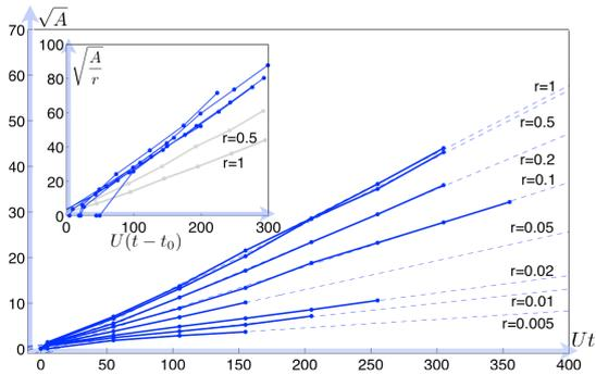
FIG. 2: Measured wave size  $L = \sqrt{A}$  growing in time for several density ratios. We observe an algebraic growth of the wave. The speed of growth depends on the density ratio  $r$ : the lighter the gas, the slower the growth. As inset, we scale the growth with the law in square root of  $r$  according to the theoretical analysis  $L \propto \sqrt{r}Ut$ . The wave shapes for  $r \neq 1$  are shown in figure 4.
