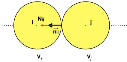
**Figure 1:** Contact  $ij$  between particles  $i$  and  $j$ , transmitting the normale force  $N_{ij}$  following the normal contact vector  $\vec{n}_{ij}$ , defining the contact's referential. The grains relative velocity at contact  $v_{ij} = v_i - v_j$  (or contact velocity) is positive when the contact is opening, and negative when the contact is further closing.
