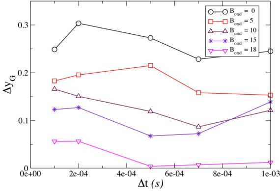
**Figure 5:** Vertical slump  $\Delta y_G$  (equation (11)) as a function of the computational time step  $\Delta t$  for 5 values of the  $B_{ond}$  number.
