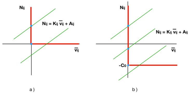
**Figure 2:** Non-smooth contact graphs for the normal forces: forces are transmitted only at contact (no distant interaction) while respecting a hard core repulsion (no inter-penetration). Non-cohesive (a) and cohesive (b) cases are represented;  $-C_0$  denotes the cohesive force threshold. In each case, all possible intersections with equation  $N_{ij} = K_{ij}\bar{v}_{ij} + A_{ij}$  (5) are shown. Blue dots show the corresponding value of the force.
