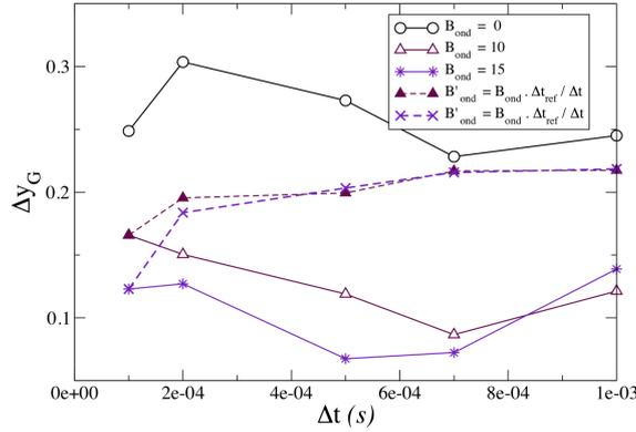
**Figure 7:** Vertical slump  $\Delta y_G$  (equation (11)) as a function of the computational time step  $\Delta t$  for 3 values of the  $B_{ond}$  number, for a cohesive threshold introduced in terms of force ( $C_0$ ) or in terms of impulse ( $I_0$ ).
