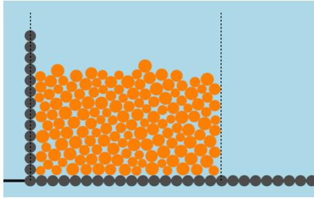
**Figure 3:** Pile counting 150 grains is its initial state, allowed to collapse in the gravity field at  $t = 0$ . Dashed lines materialise the transitory container in which the sample is created by random pluviation, before being removed so that the sample is left free to move unconfined. The darker grains are fixed and form a rough wall and plane.
