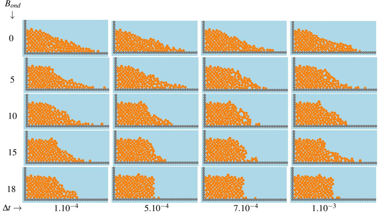
**Figure 4:** Final state of the pile after being allowed to slump under gravity for 5 values of the  $B_{ond}$  number (0, 5, 10, 15 and 18) and for four different values of the computational time step  $\Delta t = 1.10^{-4}s$ ,  $\Delta t = 5.10^{-4}s$ ,  $\Delta t = 7.10^{-4}$  and  $\Delta t = 1.10^{-3}$ .
