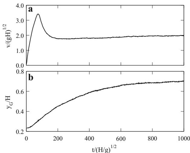
**Fig. 2** **a** Mean flow velocity  $v$  (normalized by  $\sqrt{gH}$ ) and **b** position of the center of mass of large grains  $y_G$  (normalized by  $H$ ) as a function of time (normalized by  $\sqrt{H/g}$ ) for the flow shown in Fig. 1, i.e.  $\Phi = 0.3$  and  $\theta = 22^\circ$ . The complete flow duration is 180s
