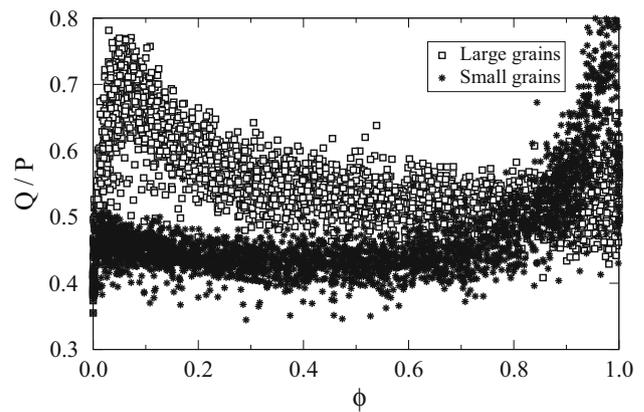
**Fig. 3** Local value of the ratio of the stress deviator to the pressure for the phase of large grains  $q_L/p_L$  and the phase of small grains  $q_S/p_S$  as a function of the local volume fraction of large grains  $\phi$ , computed in the course of time at different depths in the flow
