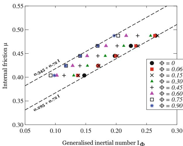
**Fig. 4** Coefficient of friction  $\mu$  of the flows as a function of the generalized inertial number  $I_\Phi$  for different flows with volume fraction of large beads  $\Phi$  varying from 0 to 0.9 and slope  $\theta$  varying between  $22^\circ$  and  $26^\circ$ . The dotted lines show affine approximations of the  $\mu(I_\Phi)$  dependence describing the increase of the static friction from 0.295 to 0.345 with  $\Phi$
