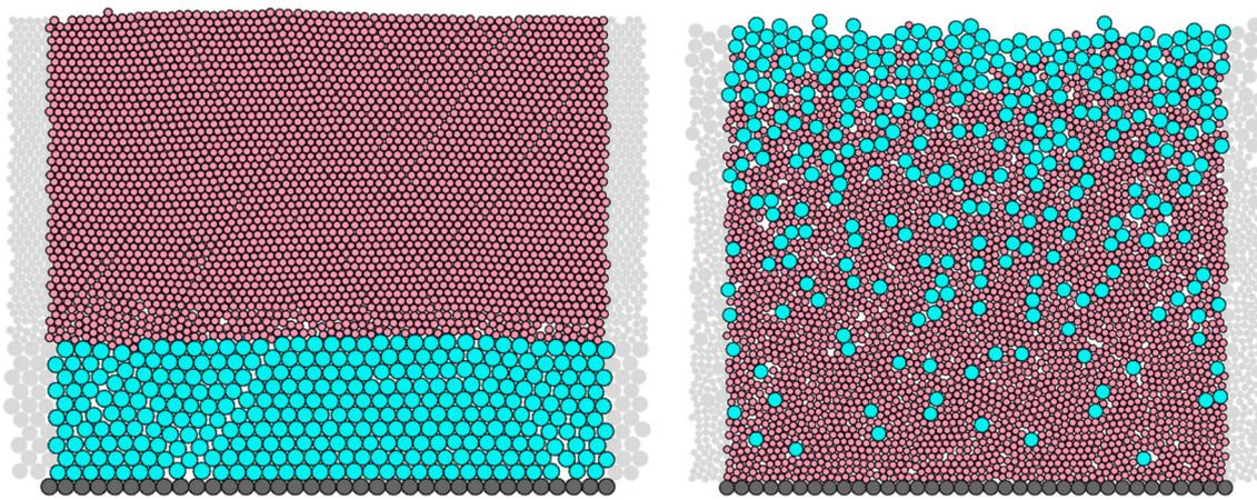
**Fig. 1** Bi-disperse granular flow with a volume fraction of large beads  $\Phi = 0.3$ , in its initial state and after steady-state is reached and segregation occurred (slope  $\theta = 22^\circ$ )
