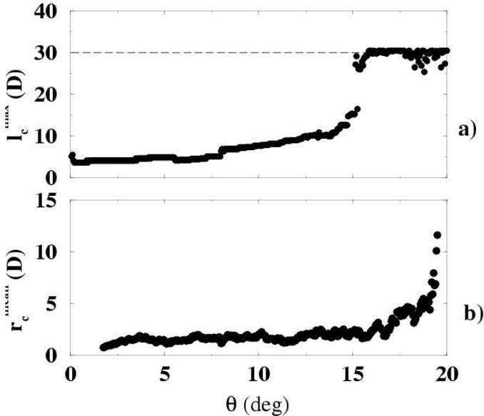
Figure 5. Evolution of the maximum size of the areas where the stress state satisfies  $\Gamma = \Gamma_c$  (graph a) and evolution of the mean size of the areas where the mobilisation of friction satisfies  $\nu = \nu_c$  (graph b) as a function of the slope  $\theta$ .
