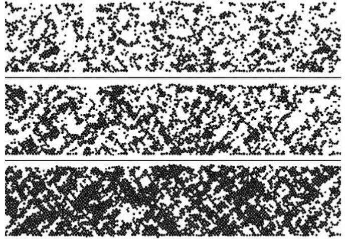
Figure 4. Snapshots of the pile for  $\theta = 0^\circ$ ,  $10^\circ$  and  $\theta_c$ . In black are represented the overloaded grains satisfying  $\gamma \geq \Gamma_c$ , where  $\gamma = q/p$  is computed from the grain moment tensor.
