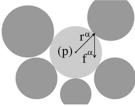
Figure 2. Grain  $p$  involved in contacts  $\alpha$  with its neighbours;  $r^\alpha$  is the vector position of the contact  $\alpha$ , and  $f^\alpha$  is the force transmitted at the contact  $\alpha$ .
