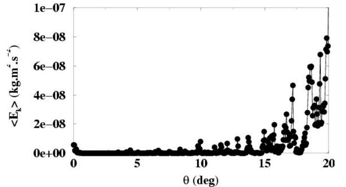
Figure 6. Mean kinetic energy of the grains as a function of the slope angle  $\theta$ . We observe increasing peaks when  $\theta \rightarrow \theta_c$ .
