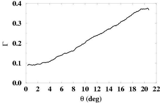
Figure 3. Evolution of the macroscopic stress ratio  $\Gamma = Q/P$  as a function of the slope angle  $\theta$ . The stability limit occurs for  $\theta = \theta_c \simeq 19.5$ , for which the stress ratio reaches the limit value  $\Gamma_c \simeq 0.36$ .
