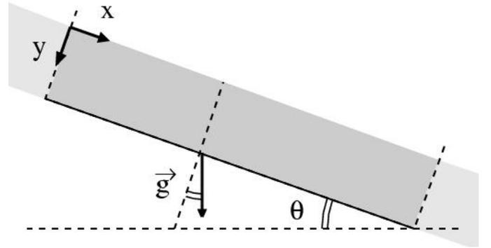
Figure 1. A periodic granular pile is driven towards stability limit by constant tilt under gravity.
