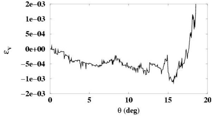
Figure 9. Variations of the packing volume  $\epsilon_V = (V - V_0)/V_0$  as a function of the slope angle  $\theta$ . We observe a period of contractant behaviour followed by dilatancy after  $\theta \approx 15^\circ$ .
