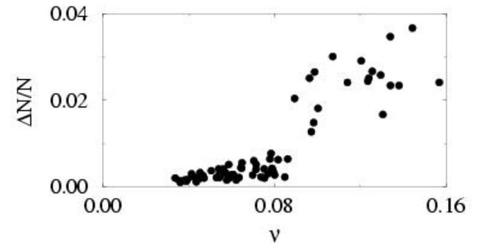
Figure 7. Size of the friction-driven instabilities as a function of the density of critical contacts  $\nu$ . We observe two different behaviours depending on if  $\nu \leq \nu_c$  or  $\nu \geq \nu_c$ , with  $\nu_c \simeq 0.08$ .
