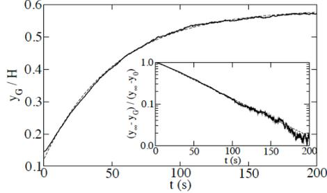
Figure 2: Position of the center of mass of the large beads  $y_G$  as a function of time  $t$  for a granular flow inclined at an angle  $\theta = 18^\circ$  and with a volume fraction of large beads  $\xi = 0.37$ . The dotted line shows the exponential fit. Inset graph: same evolution with respect to initial and final position  $(y_\infty - y_G) / (y_\infty - y_0)$  in a log-lin graph.
