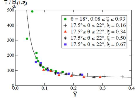
Figure 3: The normalized typical time-scale of segregation  $\bar{\tau} / \frac{H}{d_L}(1 - \xi)$  as a function of the normalized shear rate  $\|\dot{\gamma}\|$ . The plain line shows the prediction  $(1/\|\dot{\gamma}\|^2 + 75)$ .
