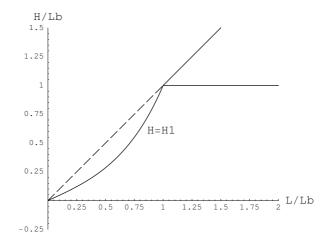
Figure 7: New version of fig.5 that includes the curve  $H_1(L/L_b)$  for  $L/L_b < 1$  where highly deflected states disappear.
