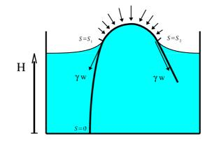
Figure 10: A lying configuration: at  $s = s_1$  and  $s = s_2$ , the interaction with the surface is modelled by discrete jumps in the inner force vector  $\boldsymbol{n}(s)$ . In the region  $s_1 < s < s_2$ , the hydrostatic pressure yields a distributed force that is continuously changing  $\boldsymbol{n}(s)$ .
