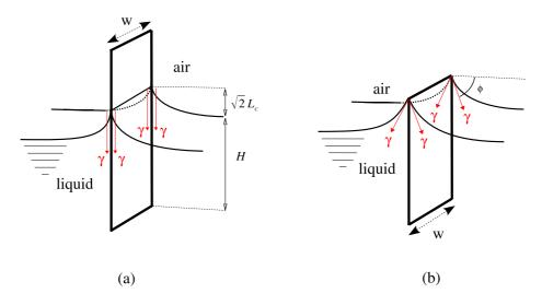
Figure 3: Elastic strip piercing (a) or only deflecting (b) a liquid surface. The (vertical) force provided by the liquid surface depends on the meniscus height.
