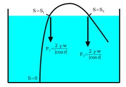
Figure 13: Twice piercing state. In the present zero capillary length approximation, left and right menisci at both crossing points  $(s_1 \text{ and } s_2)$  are replaced by point forces.
