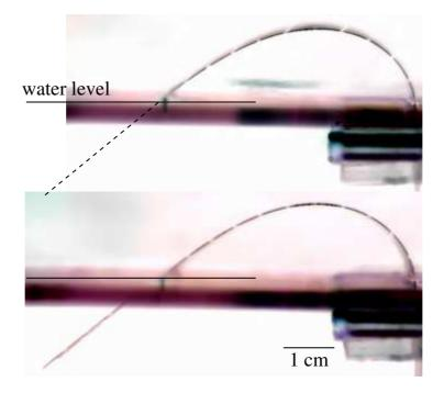
Figure 21: Free end configurations may always be lengthen without change. These two configurations with the same bath height have different lengths but an identical emerged part.
