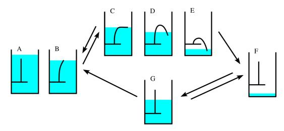
Figure 2: Sequence of experimental equilibrium states of a long strip, when lowering then increasing the bath height.
