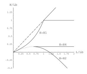
Figure 14: Extension of figure 9 where the curves corresponding to the two instabilities occurring for twice piercing states have been added (with  $L_b = 50L_c$ ). The curve  $H = H_2(L/L_b)$ , corresponding to configurations where the end of the beam emerges, connects with the curve introduced for the single piercing states (see fig.9). The dotted part of the  $H = H_2(L/L_b)$  curve is only plotted as a guide to the eye and does not correspond to any instability.
