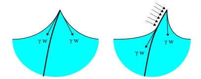
Figure 12: The two different types of configurations of lightly deflected states at non-zero  $L_c$ . Left: the two menisci joining the apex of the beam to the asymptotical bath height H are vertically symmetric. Right: the beam has a semi-submerged part.
