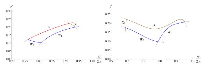
Figure 7: Islands of good knots, plotted in the parameter space of end-displacement  $z^*$  and endrotation  $\varphi$ . The end-shift is fixed at  $\delta = 0.05$ . Left: The Kirchhoff rod case, where good knots lie inside the region limited by the four curves  $S, W_1, W_2$ , and X. Right: The elastic strip case, where good knots lie inside the region limited by the four curves  $W_1, W_2, X_1$ , and  $X_2$ .
