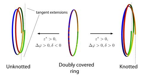
Figure 11: Beginning at the the doubly-covered ring (middle) and adding a small end-displacement, a small end-rotation and end-shift of opposite sign creates an unknotted helical-type configuration (left), while a small end-rotation and end-shift of equal sign can create a knotted configuration (right).
