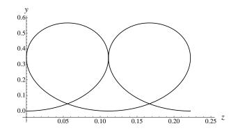
Figure 14: Self-contacting planar elastica corresponding to the limit case  $\delta \to 0$ ,  $\Delta \varphi \to 0$ , and  $z^*$  given by Eq. (6.20).
