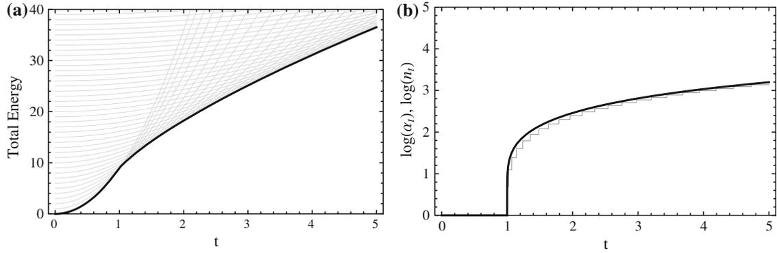
**Fig. 5** Energy and fracture density curves in the “long film” regime. *Thick lines* show the results of the limit model, they are compared with the discrete family of energies (20). The limit model can macroscopically characterize high fracture density regimes with a “damage”-like parameter
