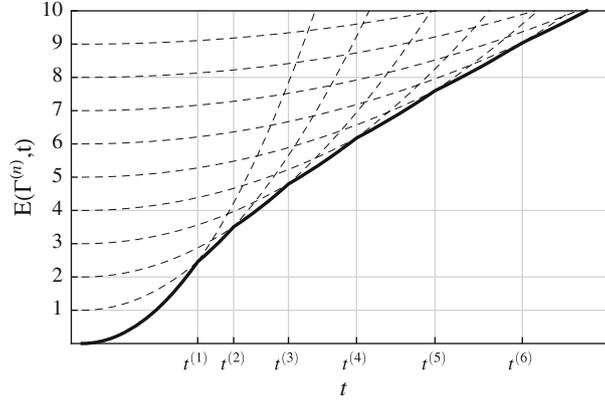
**Fig. 4** Total energy for transverse fracture without debonding for different number of cracks. The cracks are equally spaced. The optimal crack number for a given loading is that of the curve attaining the lowest energy level, this last indicated by the *continuous stroke*
