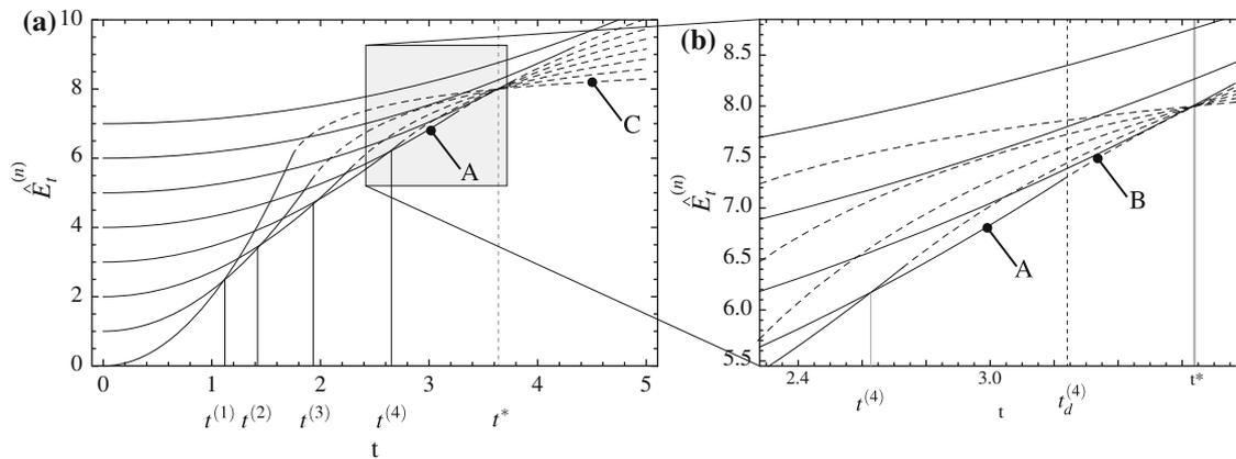
**Fig. 7** Energy curves  $\hat{E}_t^{(n)}$  with possible debonding and transverse fracture for  $\gamma = 2.2, L = 6$ . Each curve is for a specific number  $n - 1$  of transverse fractures, corresponding to the value at the intersection with the axis  $t = 0$ . The *solid continuous lines* indicate the energy is obtained for a state without debonding, the *dashed line* for a state with debonding
