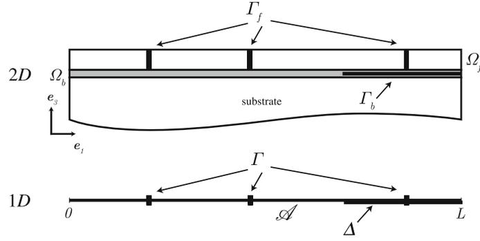
**Fig. 1** 2D: A cross-section of the 3D system: the film  $\Omega_f$  is bonded to a stiff substrate by the means of the bonding layer  $\Omega_b$ . Transverse cracks  $\Gamma_f$  debonding cracks  $\Gamma_b$  may develop in the film and in the bonding layer. 1D reduction: in the reduced uniaxial elastic bar of axis  $\mathcal{A}$ , transverse and debonding cracks are identified with  $\Gamma$  and  $\Delta$
