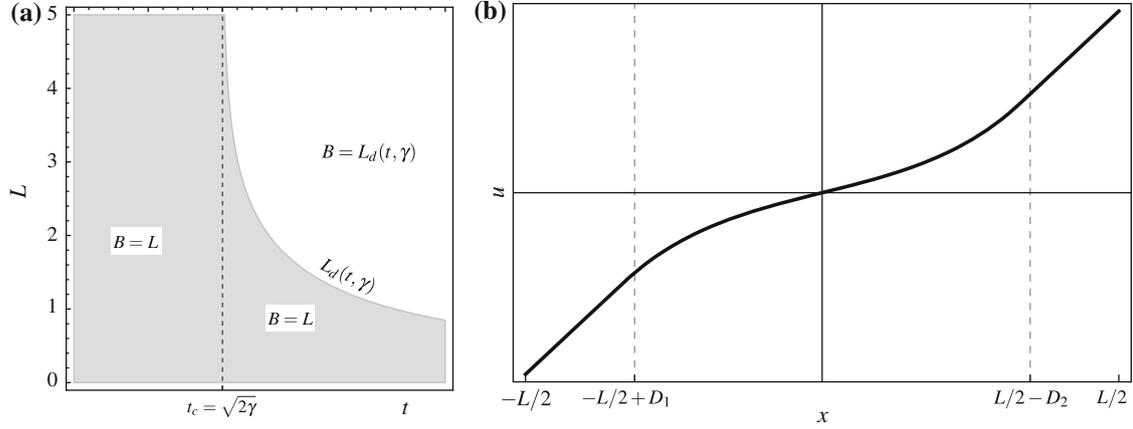
**Fig. 6** Solution of (GM) for a film with debonding and without transverse fracture. **a** Phase diagram of the optimal size of the bonded domain, as function of the film length and load intensity, where  $L_b(t, \gamma)$  is given in Eq. (33). **b** Displacement field for the partially bonded film, see Eq. (28)
