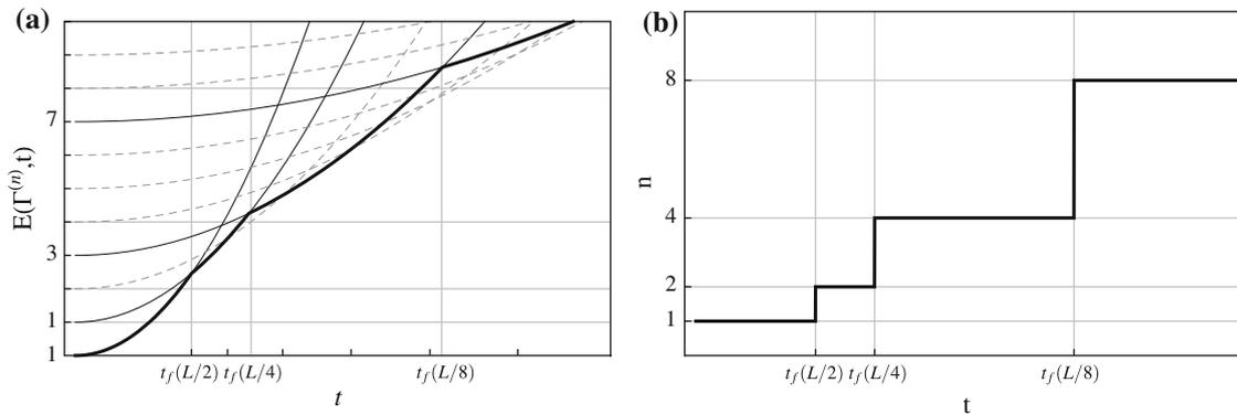
**Fig. 10** Quasi-static evolution without debonding: **a** energy curves  $E(\Gamma^{(n)}, t)$  versus  $t$  for different  $n$ , where the *thick solid line* denotes the global minimum corresponding to the solution of the evolution problem; **b** number of parts  $n_j$  of length  $L/n_j$  versus  $t$  formed by the  $n_j - 1$  equally spaced cracks, with  $n_j = 2^j$
