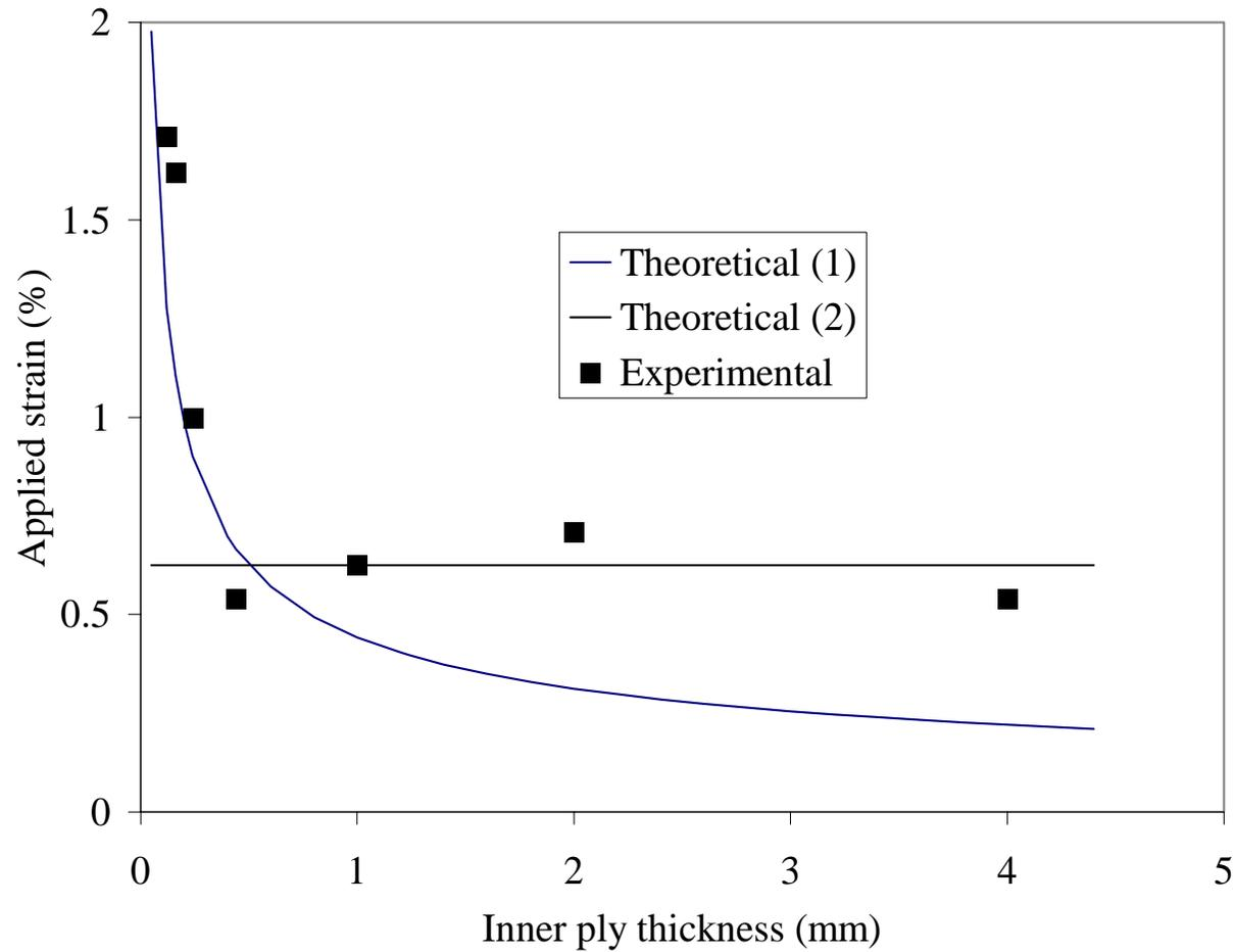
Applied strain at onset of the first micro-crack in the transverse ply *vs.* inner ply thickness.
