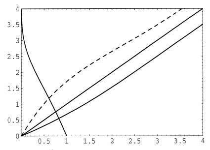
Fig. 4. The ordinate is physical here  $(y/x^{1/3})$ , in abscissa the temperature profile g (decreasing from 1–0), the velocity profile near the bottom wall  $f'/(1+\theta g)$  (dashing), the Poiseuille profile  $(yx^{-1/3})$  (straight line) and the velocity profile at the top wall  $f_h$  (plain). (No gravity, non-linear self-similar result, the profiles are plotted for the arbitrary value  $\theta = 1$ .)
