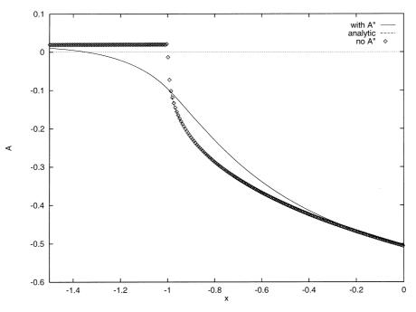
Fig. 6. The opposite of the displacement of the streamlines: A(x) comparison of the Fourier (FFT) code with and without transverse pressure variation in the Main Deck (with A'', no A'') and the self-similar solution (merged with the FFT solution). The displacement is upward (A is negative) when there is no gravity.
