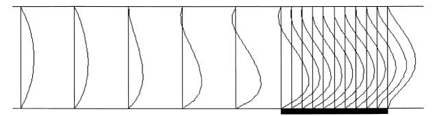
Fig. 12. Longitudinal velocity profiles computed by Fluent in a heated pipe with gravity. Notice the back flow at the upper wall induced by the heating and the increase of skin friction on the susceptor.
