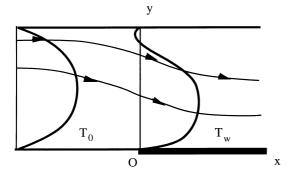
Fig. 1. The incident Poiseuille profile at temperature  $T_0^*$  encountering a heated wall at temperature  $T_w^*$ .
