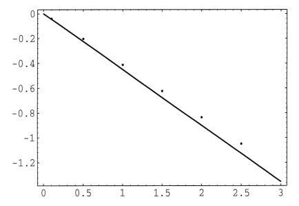
Fig. 2. Coefficient of the pressure as a function of  $\theta$ . A sudden growth of temperature promotes a pressure decrease (no gravity). Points are the non-linear self-similar results, the line is the linearized one.
