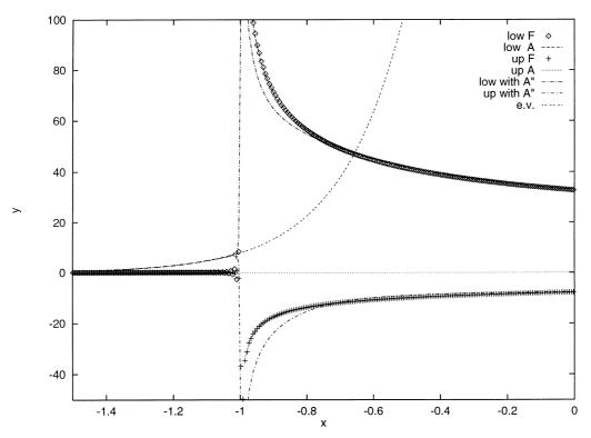
Fig. 11.  $\tau(x)$ , comparison of the Fourier code without (low *F* means Fourier solution in the Lower Deck and low *A* means analytic solution in the Lower Deck) and with (low with *A''* means Fourier solution with *A''* in the Lower Deck) transverse pressure in the Main Deck and the self-similar solution. The eigenvalue solution is plotted here too and referred to as *e.v.* The strong gravity effect may cause a separation at the upper wall, whereas the shear is increased at the lower wall.
