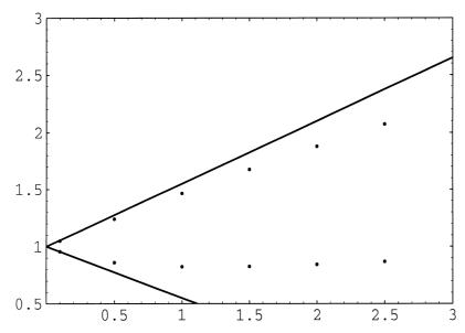
Fig. 3. Coefficient of the skin friction at the top wall  $f'_{\rm h}(0)$  (dots, greater than one), the Gittler linearized result (upper line) and the friction at the lower wall  $f''(0)/(1+\theta)$  (dots, lower than one) as a function of the relative increase of temperature  $\theta$  (no gravity, self-similar and non-linear).
