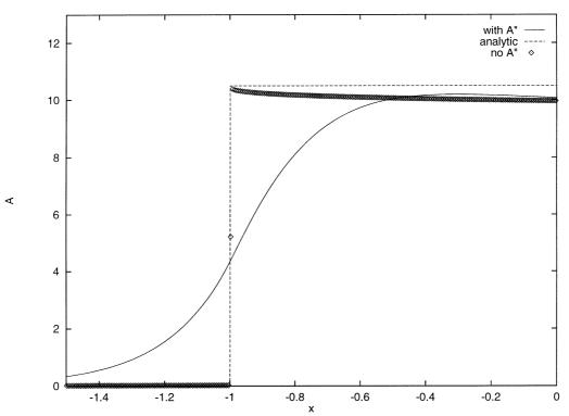
Fig. 9. The opposite of the displacement of the streamlines: A(x), comparison of the Fourier code with (with A'') and without (no A'') transverse pressure in the Main Deck and the self-similar solution (analytic). The displacement is downwards when there is strong gravity.
