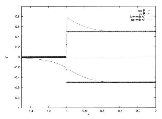
Fig. 8. Perturbation of skin friction (no gravity case) low (resp. up) *F* means a Fourier solution in the (resp. Upper) Lower Deck without *A*". The perturbation increases on the upper wall (positive value) and decreases on the lower one (negative value). *A*" induces upstream influence: a decrease of  $\tau$  in the two decks (for x < -1).
