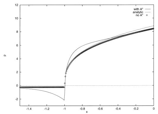
Fig. 10. P(x), comparison of the Fourier code with and without transverse pressure in the Main Deck and the self-solution.
