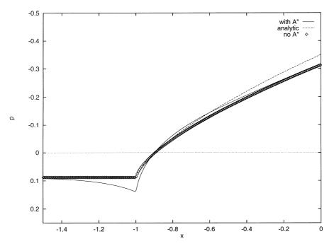
Fig. 7. The pressure P(x), comparison of the Fourier code with and without transverse pressure in the Main Deck and the self-similar solution. The heating promotes a pressure drop.
