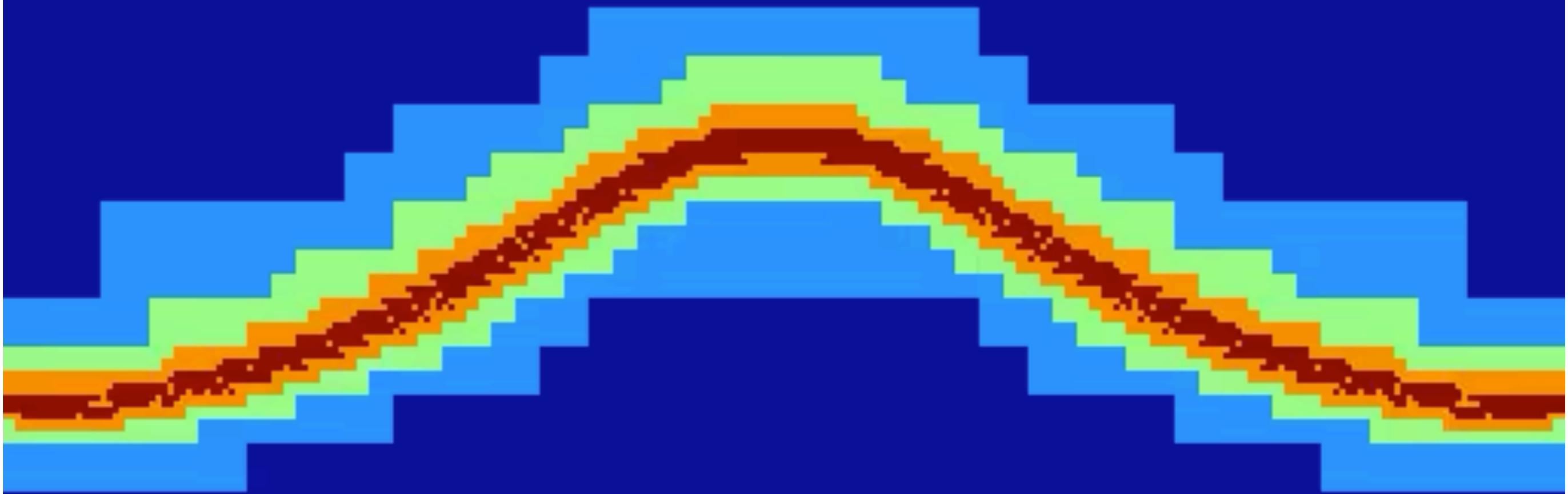
**breaking wave: automatic adaptative mesh at the "singular interface"**
