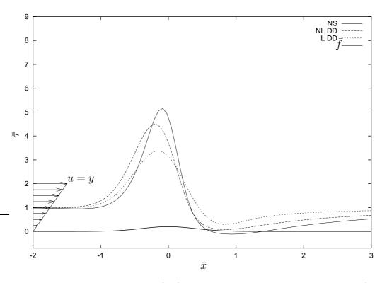
Fig. 2. Comparing Navier Stokes (NS), non linear full Double Deck equations (NL DD), and linearized Double Deck equations (L DD),  $\alpha = 2$ , Re = 1000.
