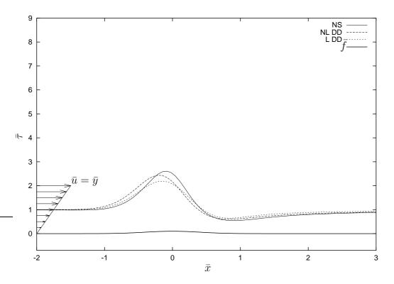
Fig. 1. Comparing shear stress for Navier-Stokes (NS), non-linear full Double Deck equations (NL DD), and linearized Double Deck equations (L DD),  $\alpha = 1$ , Re = 1000. The three descriptions are similar for  $\alpha < 1.5$ .
