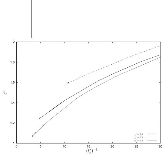
Fig. 8. The selfsimilar relation between the mass  $\bar{m}$ , the inverse of the saturation length  $l_s^* = \bar{l}_s \bar{m}^{-3/4}$ , and the velocity  $c^* = \bar{c} \bar{m}^{1/4}$  of the "dune" for three values of the threshold:  $\tau_s^* = 0.9$ , 0.8, and 0.5. For a fixed threshold, there is a maximal value of the saturation length  $l_s^*$  over which there is no solution.
