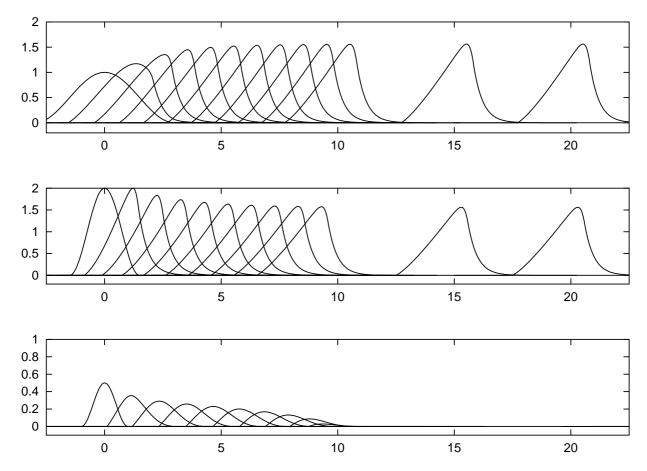
Fig. 4. The non-linear Double Deck evolution of three "dunes", for  $\bar{t} = 0, 1, 2, ..., 10$ ,  $\bar{t} = 15$ , and  $\bar{t} = 20$ . Two upper curves:  $\bar{m} = 3$  is conserved,  $\bar{\tau}_s = 0.9$ , and  $1/\bar{l}_s = 2.5$ , but two different initial shapes leading to the same final solution. Lower curve:  $\bar{m} = 0.5$ ; when the initial mass is too small, the "dune" is washed, it loses mass.
