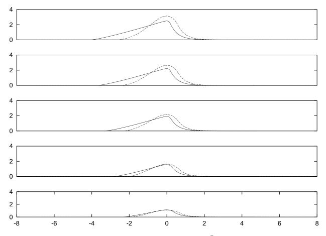
Fig. 6. The non-linear final moving "dune" solution  $\bar{f}_{fin}(\bar{x} - \bar{c}\bar{t})$  is represented with solid lines, the linear solution is represented with dashed lines, and  $\bar{\tau}_s = 0.9$ ,  $1/\bar{l}_s = 2.5$ ,  $\bar{m} = 2, 3, 4, 5, 6$  (bottom curve to top curve).
