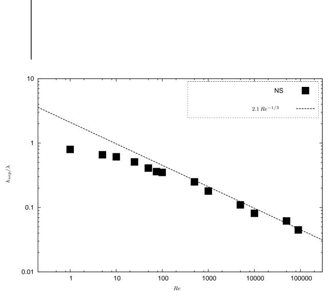
Fig. 3. Value of the relative height of the gaussian bump at incipient separation. Comparing full numerical Navier-Stokes (squares) and the prediction from the non linear Double Deck equations (line). The asymptotic theory well predicts the hight of incipient separation.
