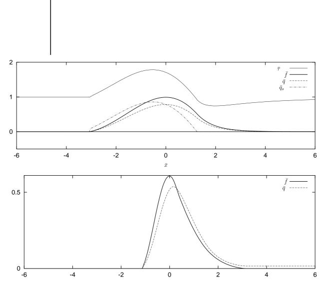
Fig. 5. Two linear Double Deck examples of model dune in the moving frame,  $\bar{\tau}_s = 0.9$ , and  $1/\bar{l}_s = 1.5$ . On the upper curve  $\bar{m} = 3$  is conserved, plot of the skin friction, associated saturated flux and value of the actual flux. On the lower curve,  $\bar{m} = 1$ , plot of the skin friction, and value of the flux  $\bar{q}$ . The non zero value of  $\bar{q}$  after the end of the model dune shows that there is loss of mass.
