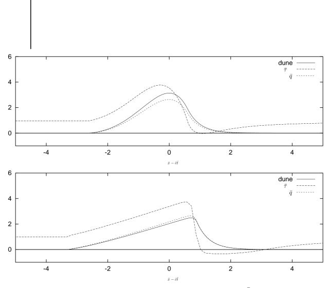
Fig. 7. An example of a final moving "dune" solution ( $\bar{\tau}_s = 0.9, 1/\bar{l}_s = 2.5, \bar{m} = 6$ ). Upper curve, the linear case. The extrapolated skin friction is slightly negative. Lower curve, the non-linear case: the stoss side is nearly flat. The skin friction is represented; it is negative in the lee side: there is boundary layer separation.
