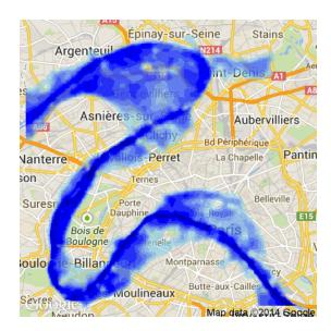
Figure 4: A figure generated from simulation at t = 120000s showing the inundated area in 1910
