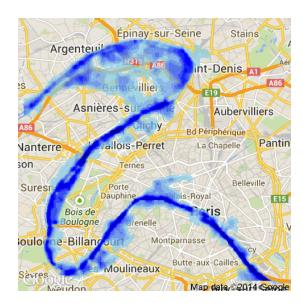
Figure 6: A figure generated from simulation at t = 120000s showing the inundated area in 1982
