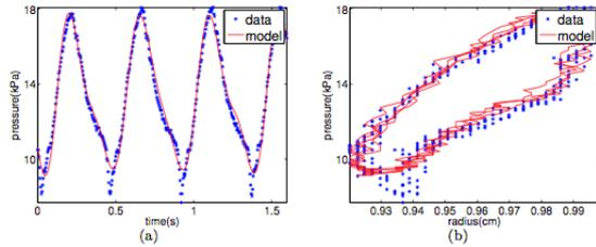
Figure 1. One case of comparison between data (star) and the fitted model (red line) at the location MD: the time series of pressure (a) and the hysteresis loop of radius and pressure (b).
