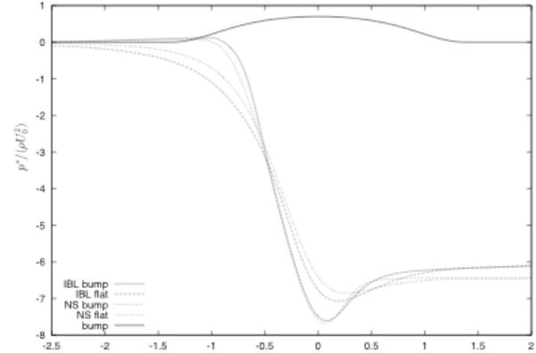
Fig. 2. Comparison of integral (IBL) and Navier Stokes pressures. The IBL well predicts the effect of asymmetry in the flow.
