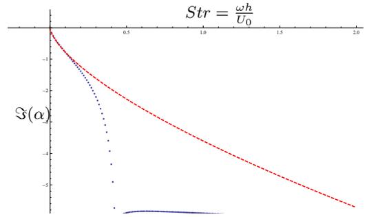
Figure 13: Imaginary part of  $\alpha$  as a function of  $Str$ , given by a numerical resolution of the Rayleigh equation with a Poiseuille flow (dots), the solution for a top-hat jet is also represented (dashed line)
