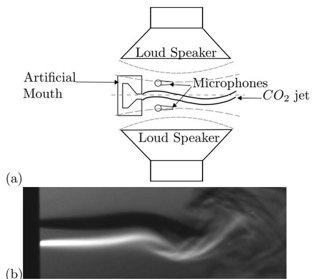
Figure 1: (a) Experimental setup used for the flow visualisations; (b) example of a visualisation with the setup
