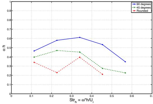
Figure 8: Evolution of the parameter  $\alpha h$  with the Strouhal number for the three simulated configurations
