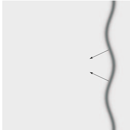
FIG. 4. Transverse sinusoidal modulation of the soliton. We represent the modulus of the wave-function. The longitudinal stretching near the inflection points creates modulated depth, then modulated velocity and formation of trough which slow down even more.
