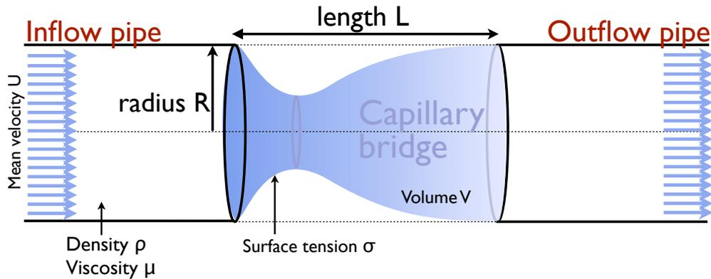
FIGURE 1. Sketch of the flow configuration: a capillary bridge held between two pipes with a throughflow.
