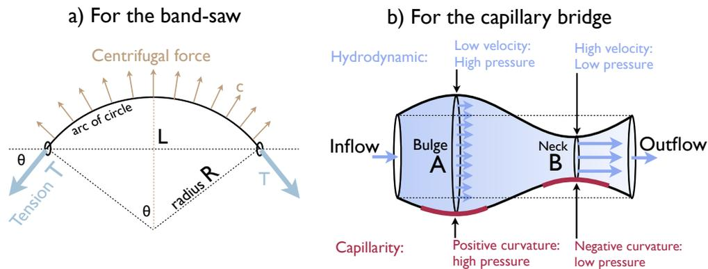
FIGURE 3. Sketch for the Band-saw instability and the analogy with the dynamic instability of the capillary bridge.
