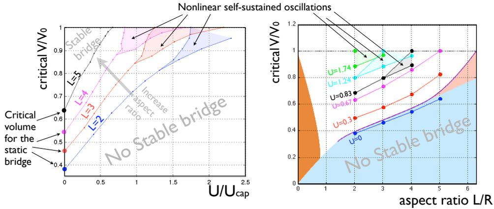
FIGURE 8. Overview of the dynamic behaviour of the simulations of the Navier-Stokes equations.
