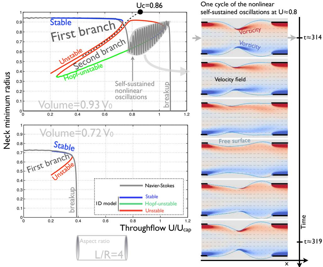
FIGURE 6. Comparison of the bifurcation diagram for the 1D nonlinear model of Eggers & Dupont (1994) and Navier-Stokes simulations. For these simulations,  $\nu = Oh = 0.01$ . For a volume close to 1, we observe nonlinear self-sustained oscillations corresponding to a saturated Hopf instability, and for a low volume, breakup of the bridge.  $U_c$  indicates the critical velocity for the cylindrical case from (2.1).
