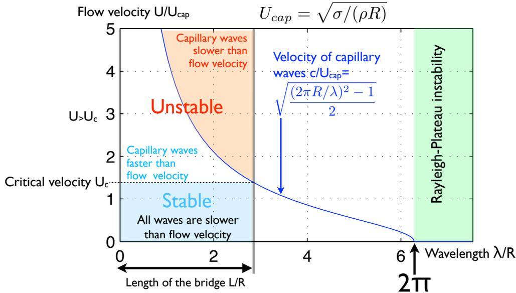
FIGURE 4. A sketch showing how the Rayleigh-Plateau instability is a particular case of the instability of the bridge with throughflow. For simplicity we have used the dispersion relation valid for long waves from §3.1 which we have used in the paper. For the full dispersion relation, see for instance Rayleigh (1879); Chandrasekhar (1981).
