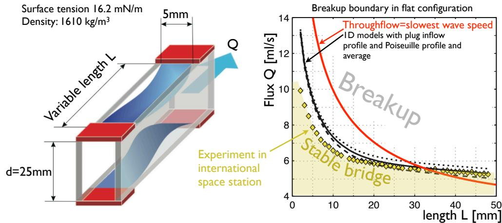
FIGURE 9. Figure adapted from the microgravity experiment of Conrath *et al.* (2013). The line where the throughflow is equal to the slowest capillary wave speed corresponds to our theory.
