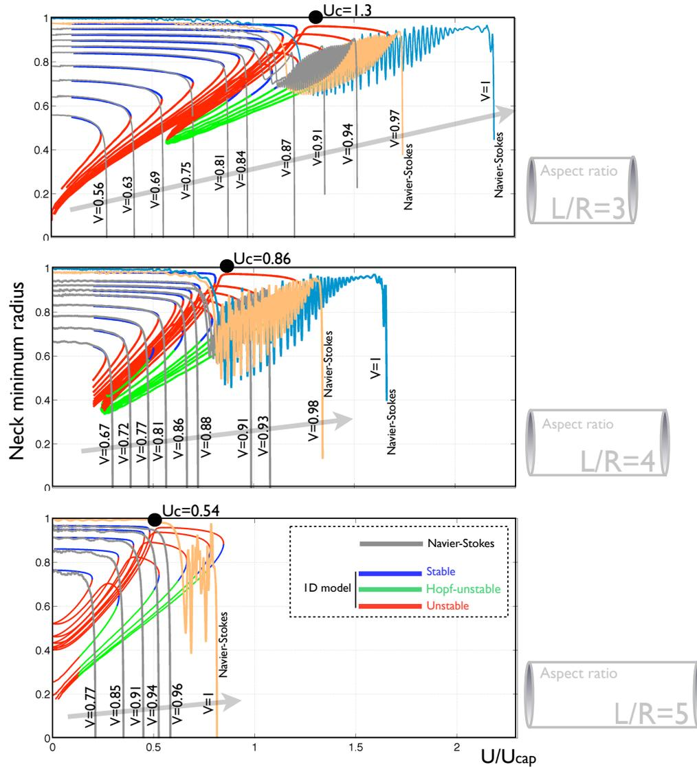
FIGURE 7. Overview of the numerical simulations and bifurcation diagrams of the capillary Venturi. We see the breakup and the self-sustained oscillations.  $U_c$  indicates the critical velocity for the cylindrical case from (2.1). For these simulations  $\nu = Oh = 0.01$ .
