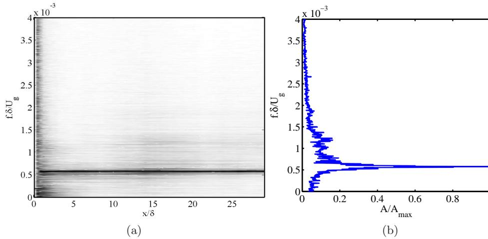
Figure 6: a) Experimental spectrum as a function of the downstream position for  $U_g = 20$  m/s and  $M = 3.7$  and splitter plate thickness  $e = 2.2$  mm. The maximum frequency remains unchanged with the distance; b) Spectrum at  $x/\delta_g = 20$ .
