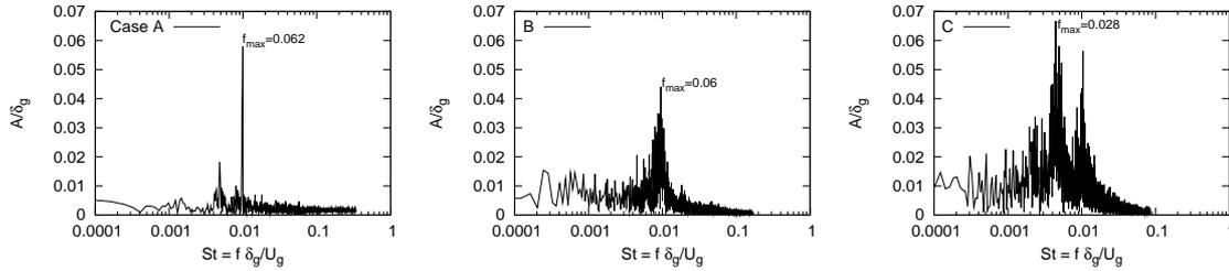
Figure 16: Simulation results. FFT of the position of the interface at  $x/e = 8$  and  $M=20$ ,  $r = 10$ .  $e/\delta_g = 0.5, 1, 2$  (from left to right). The forcing frequencies are not visible. The peak observed in the spectrum is more noisy for large  $e/\delta_g$  ratios.
