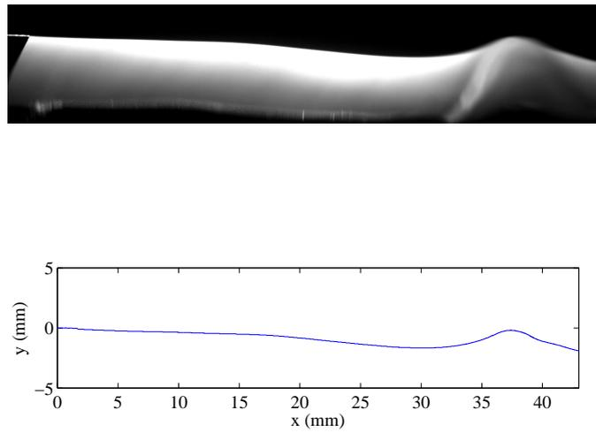
Figure 4: Top: Laser slice of the flow seeded with fluorescein. The white line on the left is a reflection on the upper surface of the splitter plate. Bottom: Interface extracted from the image:  $U_g = 10$  m/s and  $U_l = 0.35$  m/s.  $e = 0.2$  mm.
