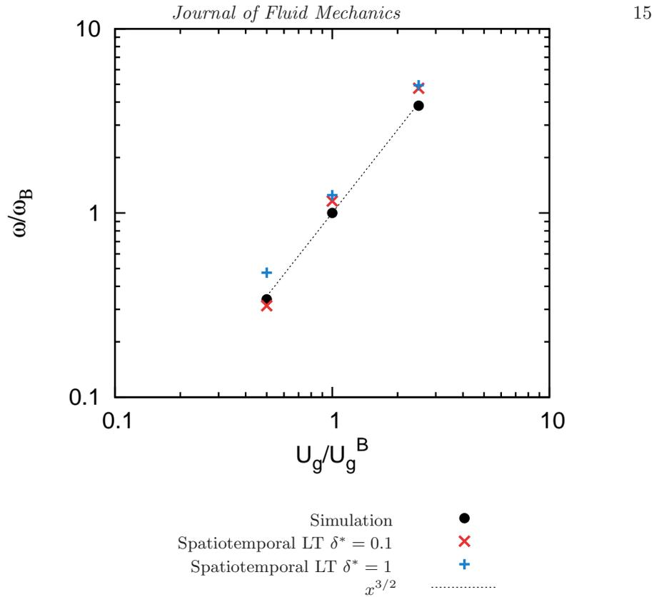
Figure 13: Peak frequency as a function of the gas velocity at large dynamic pressure ratios.  $U_g^B$  represents the gas velocity previously used to perform the simulations at constant gas velocity (Table 1) and  $M = 20$ .  $\omega_B$  is the observed frequency at these conditions.
