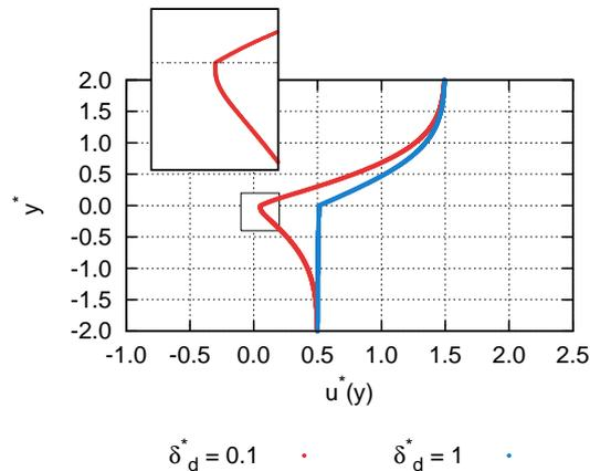
Figure 7: Example of the base flow profile used for the temporal and spatiotemporal calculations for  $\Delta U^* = 0.5$ ,  $m = 0.012$  and  $\delta_l^* = 1$ .
