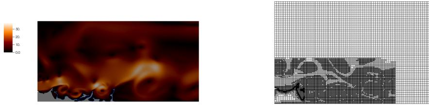
Figure 18: Left: Simulation domain and velocity norm field (m/s). Right: Spatial mesh distribution (the view has been zoomed to appreciate the different grid levels).
