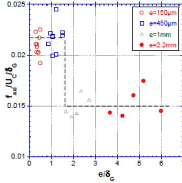
Figure 15: Experimental peak frequency as a function of the ratio  $e/\delta_g$  at  $M = 16$ . The measurements are taken at  $x = 5$  mm. Results extracted from Ben Rayana (2007).  $U_c$  stands for the Dimotakis velocity  $U_D$  (Eq. 5.3).
