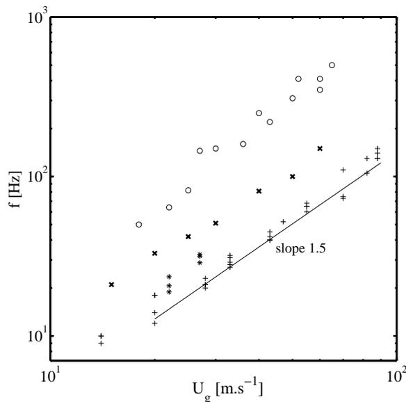
Figure 1: Experimental frequency vs. gas velocity for various sets of experiments with  $M > 4$ . (+) Data obtained by Raynal (1997)  $M = [4.2 : 2115]$ , (o) Marmottant & Villermaux (2004)  $M = [4 : 108]$ , (x) Ben Rayana (2007)  $M = 16$  and (\*) Matas *et al.* (2011)  $M = [5 : 14]$ . The most unstable frequency is shown to scale as  $U_g^{3/2}$  for large  $M$ .
