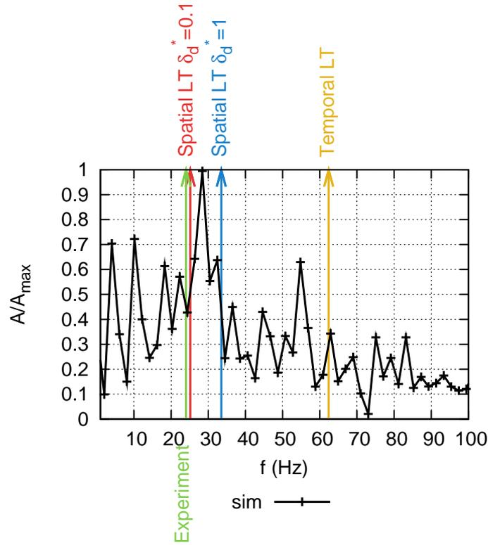
Figure 20: Fourier analysis of the interface height temporal evolution at  $x/\delta_g = 11$  obtained from numerical simulation, experiments and theoretical predictions by a temporal analysis and spatiotemporal analysis. Conditions of table 3.
