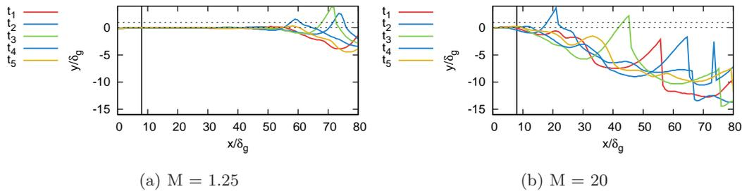
Figure 9: Interface position sampled at different times during one cycle ( $\Delta t^* = 3750$ ). The axis have been stretched to facilitate the visualization. The vertical line represents the location where the interface is sampled to obtain the FFT.
