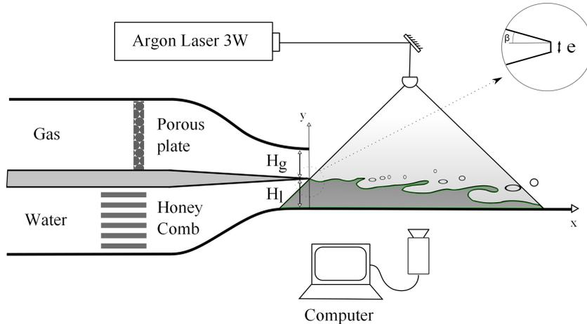
Figure 2: Sketch of the experimental set-up. Two splitter plates are used in the experiment:  $e = 0.2$  mm and  $\beta = 4.15^\circ$ , and  $e = 2.2$  mm and  $\beta = 4.1^\circ$ .
