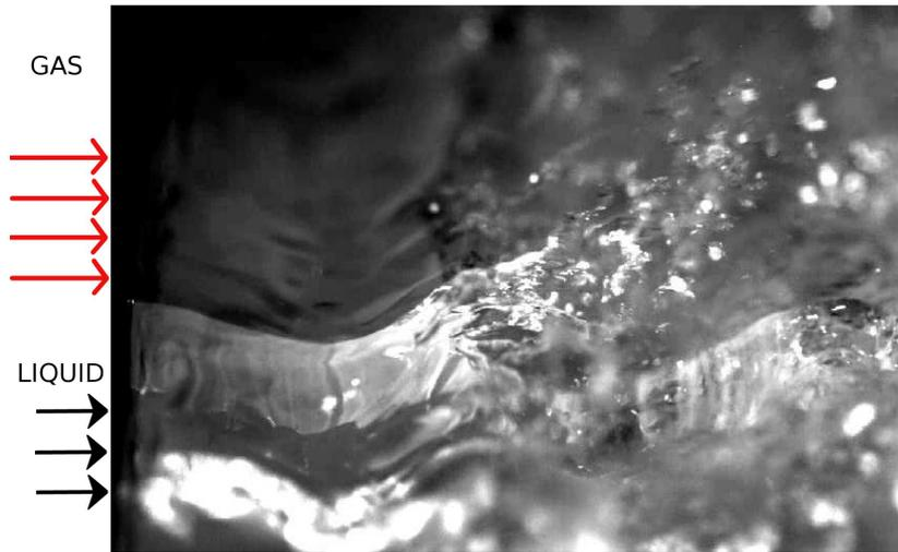
Figure 3: Visualization of the shear instability with both a laser slice and white light:  $U_g = 25$  m/s and  $U_l = 0.55$  m/s.  $e = 0.2$ mm.
