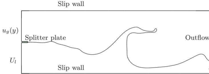
Figure 8: Computational domain and boundary conditions for the simulations at low density ratios ( $r = 0.1$ ).
