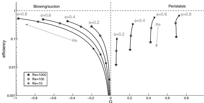
FIGURE 6. Flux and efficiency of pumping while varying the Reynolds number  $Re_w \in [1, 1000]$  (solid line), and the actuation amplitude  $\phi$ , for  $L = 2\pi$ . Note that the case  $Re_w = 1$  is not represented by an additional symbol.
