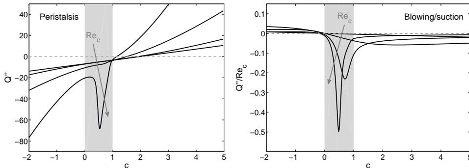
FIGURE 10. Wall actuation interaction with base flow: pumping flux as a function of the wavespeed  $c$  for  $Re_c = 1, 10, 100, 1000$ . The parameter range where a critical layer is present  $c \in [0, 1]$  is highlighted by a shaded strip.
