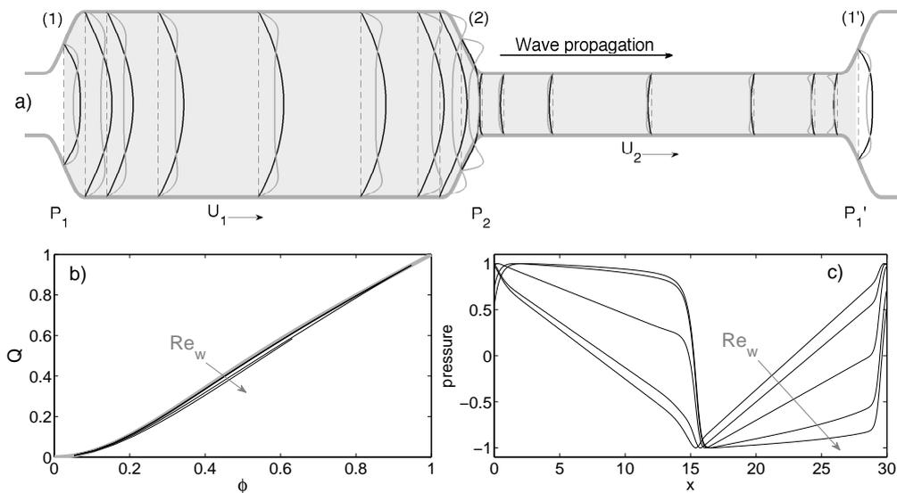
FIGURE 2. Configuration of the peristaltic pumping model (2.6). a) Velocity profiles for  $\phi = 0.5$ , wavelength  $L = 30$  and  $Re_w = 1$  (black) and  $Re_w = 1000$  (light gray). For  $Re_w = 0.1, 1, 10, 100, 1000$ : b) the flux  $Q$  as a function of the constriction  $\phi$ , and c) the centerline pressure along one wavelength, normalized to the amplitude range  $[-1, 1]$ .
