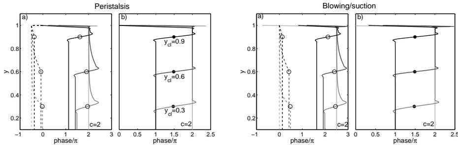
FIGURE 9. a) Phase of  $\hat{u}_y$  (plain)  $\hat{v}$  (broken) and b) departure from quadrature:  $\text{phase}(\hat{u}_y) - \text{phase}(\hat{v}) - \pi/2$ , at  $Re_c = 10^6$  for  $c = 2$  (light gray), and for wavespeeds such that the critical layers are at  $y_{cl} = 0.3, 0.6, 0.9$  (from gray to black). The position of the critical layer is shown with the symbols.
