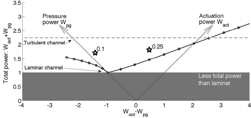
FIGURE 8. An alternative representation of the "power plane". Here the axes are rotated such that horizontal lines correspond to constant total power  $W_{act} + W_{pg}$ . The dotted line represents the power balance for blowing and suction for a fixed flux  $Q$ , at  $Re_w = Re_c = 2000$ . The two stars are the turbulent control results of Min *et al.* (2006) with wave amplitude 0.1 and 0.25.
