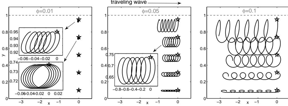
FIGURE 5. Trajectories of five particles at  $Re_w = 100$ ,  $L = 10$  for 6 periods, with three wave amplitudes  $\phi = 0.01, 0.05, 0.1$ . Stars locate the particles initial position. The motion of flow particles is shown in the movies available with the online version of this paper.
