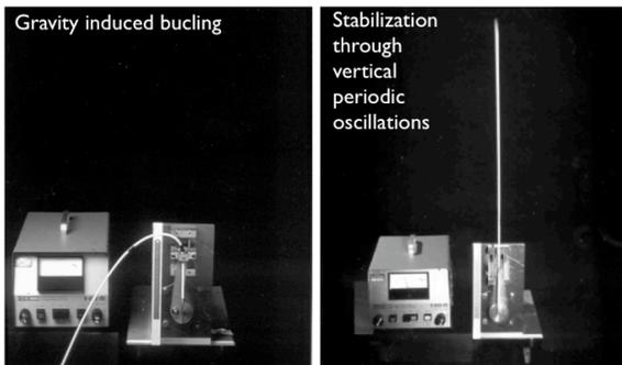
Figure 7: The "indian wire trick". A wire is held clamped upwards. a) without excitation the wire buckles under its own weight and falls down on the side, whereas in b), the attachment point is oscillated vertically and the upward position is stabilized. Figure from [16]. This example shows how a periodic excitation can stabilize an elastic system by making use of its elastic properties of oscillations.
