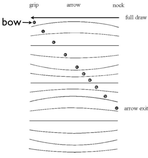
Figure 5: The Archer's paradox. Dynamic bending of the arrow right after being released from the archer's finger. The arrow oscillates and this oscillation must be tuned such as to avoid collision with the bow. Figure from [12].
