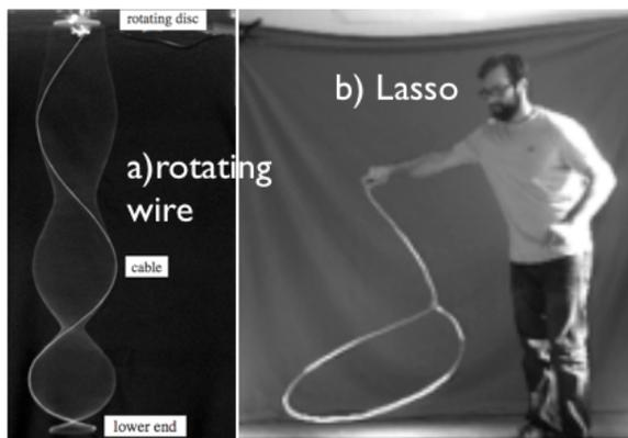
Figure 8: a) A wire in a rotating frame may adopt different steady configurations under the effect of the centrifugal force: a force that depends on the position of the wire with respect to the axis of rotation. b) The steady shape of the lasso. Figure adapted from [18] and [19].
