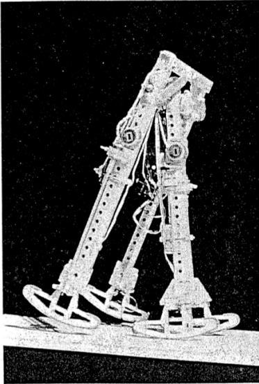
Figure 2: Biped used for experiment on two-dimensional gravity-powered walking. Figure from [3]. These studies are ideal illustrations of motion at almost constant energy. We make use of gravity potential energy and elastic potential energy in our bodies to approach this ideal of a motion at constant energy.
