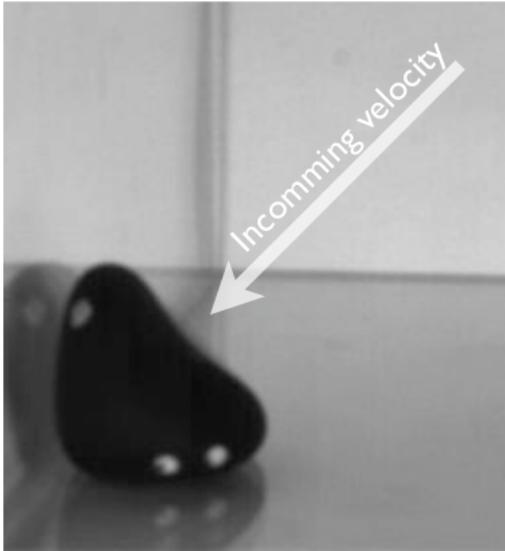
Figure 6: Impact of a squash ball right at a corner. Image from [13]. The ball shows a strong elastic deformation. The bounce at the corners leads to a large dissipation of energy, due to viscous loss in the deformation of the shell dry friction at the contact surface between the deforming shell and the surface.
