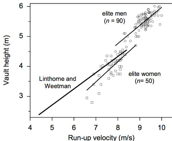
Figure 4: This plot shows the strong correlation between vault height and run-up velocity within groups of elite pole vaulters. Figure from [10]. We may at first sight think that the vault height should be proportional to the square of the run-up velocity, but we see a linear law emerging, this is the trace of energy losses at the planting shock through inelastic response of the body.
