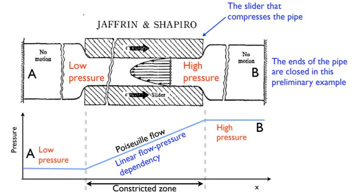
Figure 2.2: Sketch for the pumping mechanism of peristalsis. Image adapted from [Jaffrin and Shapiro, 1971].
