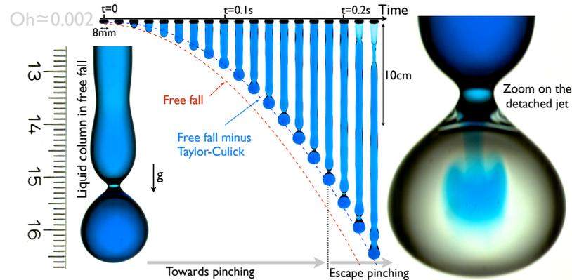
Figure 2.6: Free-falling liquid column experiment showing the escape of pinch-off.
