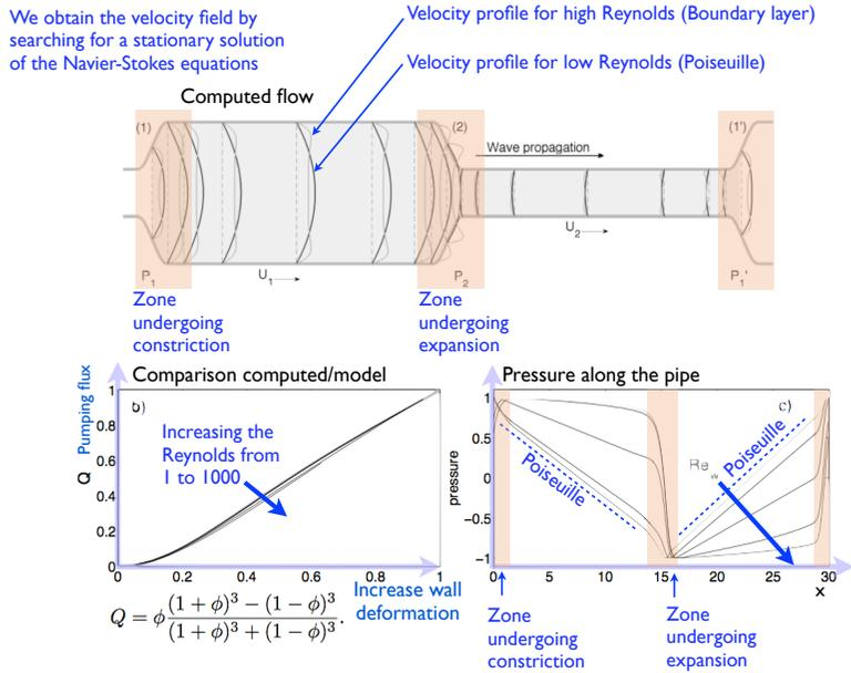
Figure 2.3: Quantitative validation of the piecewise-continuous channel for peristalsis.
