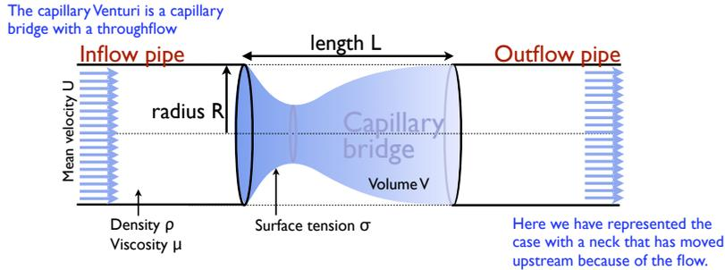
Figure 2.7: Sketch of the capillary Venturi.
