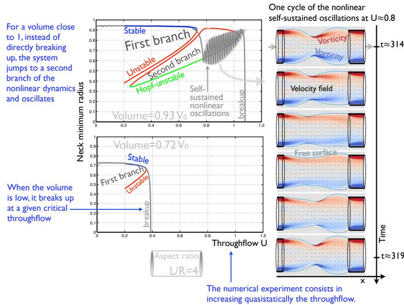
Figure 2.8: Capillary Venturi: comparison of the numerical simulations and the nonlinear branches.
