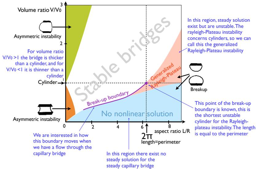
Figure 3.1: Overview of the properties of the static capillary bridge (no gravity).
