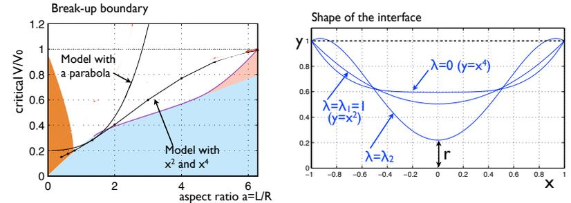
Figure 3.3: Left: Comparison of the breakup boundary with that predicted by the one degree of freedom model and the two degrees of freedom model. Right: Shapes of the liquid bridge with different values of the second degree of freedom  $\lambda$ .
