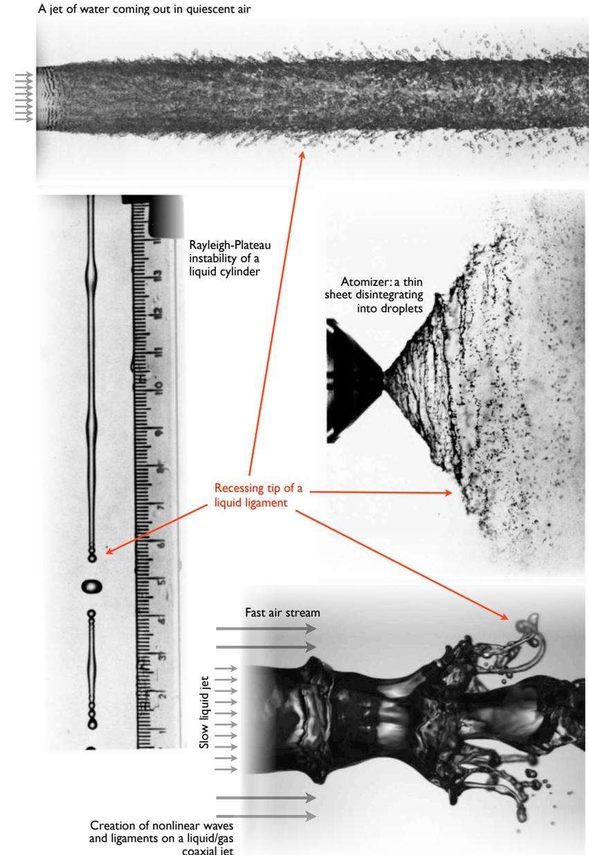
Figure 4.1: Images of creating droplets from a liquid body: atomization. All images come from [VanDyke, 1982] except the coaxial jet which comes from [Marmottant and Villermaux, 2004].
