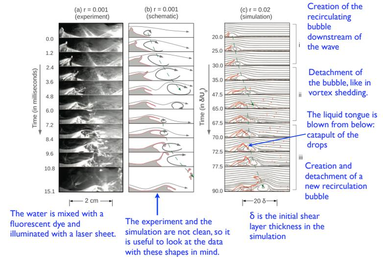
Figure 4.11: Experiments and numerical simulation for the catapult mechanism of droplets by the self-similar wave.
