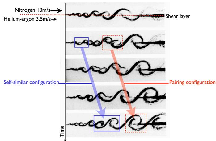
Figure 4.14: A shear layer at pressure 8 atmospheres and Reynolds 850,000. Image from [VanDyke, 1982].
