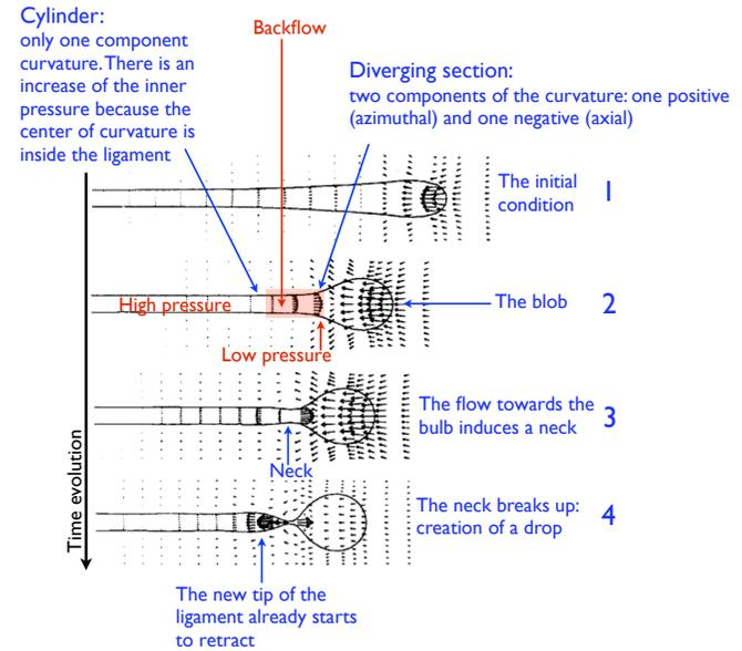
Figure 2.5: The end-pinching mechanism for creation of the neck. Image adapted from [Stone and Leal, 1989].
