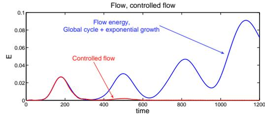
**Figure 11** Flow energy when excited with oscillating volume force in the upstream region of the shear layer with (*dashed*) and without control (*solid*). One sees the energy cycles for the uncontrolled flow. For the controlled flow, only the first growth cycle is still present: the controller has prevented the regeneration of the wave packet.
