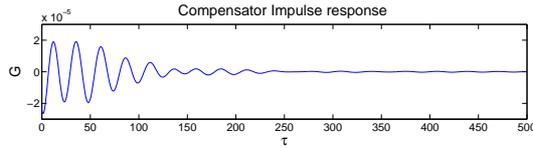
**Figure 10** Actuation signal at the output of the controller for an impulse at the measurement. Can as well be interpreted as a convolution kernel to obtain the actuation signal from past measurements.
