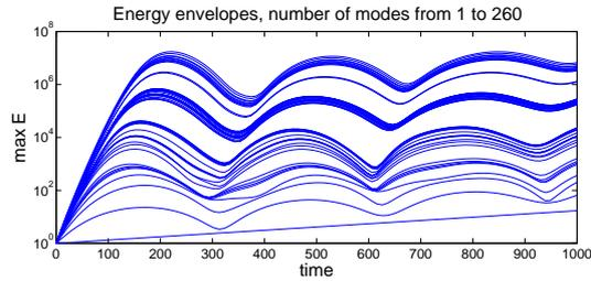
**Figure 5** Envelope of maximum energy growth from initial conditions. The different lines correspond to increasing number of eigenmodes included in the optimization, 1 to 300 from bottom to top.
