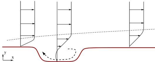
**Figure 1** Sketch of the geometry, with Blasius boundary layers upstream and downstream of the domain, with recirculation inside the cavity. The recirculating region is isolated from the free-stream by a shear layer.
