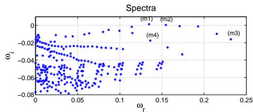
**Figure 3** Eigenvalues of the cavity flow. One sees two unstable modes with imaginary part about 0.15.
