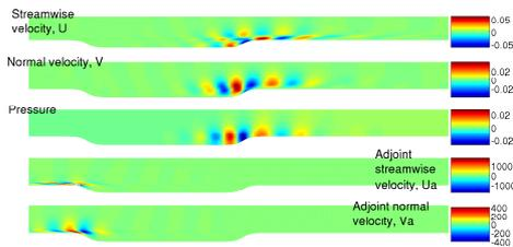
**Figure 4** Least stable eigenmode, corresponding to the eigenvalue labelled  $m1$  in figure 3. a) streamwise and normal velocity, b) pressure, c) velocity components of corresponding adjoint eigenmode
