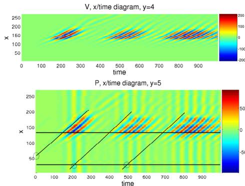
**Figure 7** streamwise/time diagram of a) the normal velocity and b) the pressure in the free-stream, at  $y = 4$  for the worst case initial condition. The propagation of the wave packet with group velocity approximatively 0.3 can be seen by the oblique rays in a) and b) , and the global changes of pressure are seen by the vertical rays in pressure b).
