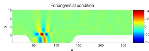
**Figure 6** The worst case initial condition for energy growth when including 200 modes in the optimization. It corresponds to time 200 of the most energetic envelope of figure 5. The initial condition is a wave packet in the upstream region of the shear layer. The wave packet is represented at time 20 of its evolution, so that its features are more easily recognizable.
