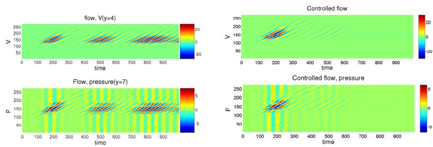
**Figure 12**  $x/t$  diagrams for the flow normal velocity and pressure in the case a) without control, and b) with control. The vertical rays of the pressure variation is still visible, but the wave packet regeneration is prevented.
