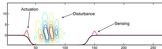
**Figure 8** Sketch of the control setting. One actuator applying blowing and suction is located at the upstream lip of the cavity, and one sensor measuring wall shear stress  $u_y$  is located at the downstream lip of the cavity. The flow is excited by a random forcing in the upstream region of the shear layer.
