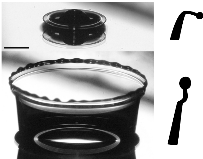
FIG. 4. (left) Images illustrating the crown sheet at 250 and 2100 \mu s after impact. (right) Cartoon of sheet cross-section. At early times, the leading edge of the sheet is almost horizontal. The shape changes as the rim retracts relative to the fluid (though still moving away from the center in the laboratory frame) and entrains the fluid in the sheet. Eventually the entire flat portion of the sheet is entrained in the rim. The kink in the late time sheet is a wave generated when the rim reaches the vertical section of the sheet. Scale bar equals 2 mm.
