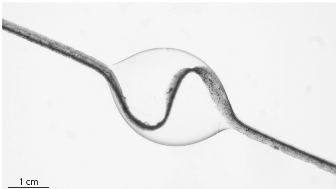
Figure 5 – Elasto-capillary buckling. Silicone oil drop sitting on a polyvinyl-siloxane fiber. When slack is given to the system, i.e. the fiber ends are brought closer, the capillary forces developed by the drop are sufficient to make the fiber buckle and coil within it.
