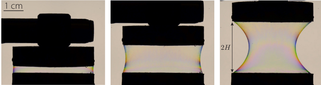
Figure 4.22 – Liquid soap film between two parallel rings adopting a catenoid shape for different ring distances 2H . It should be noted that the rings are open, therefore the pressure inside the catenoid is therefore equal to atmospheric pressure.
