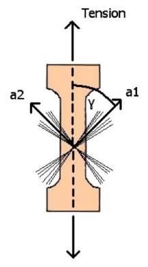
FIGURE 3. Lattice structure of crossing collagen fibres with fibre dispersion taken into account.
