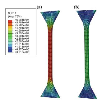
FIGURE 11. Cauchy stress in Pa of sample strained by 50% (a) Parallel to the Langer lines (b) Perpendicular to the Langer lines.
