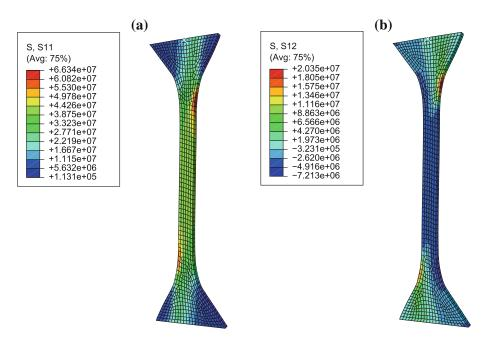
FIGURE 12. Cauchy stress in Pa of a non-symmetric sample strained by 30% (a)  $\sigma_{11}$  (b)  $\sigma_{12}$ .
