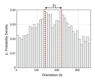
FIGURE 2. Histogram of collagen orientations. The two distinct peaks correspond to the preferred orientation of the two fiber families. The angle,  $\gamma$ , is half the distance between the two peaks i.e.  $\gamma = 41^{\circ}$ .
