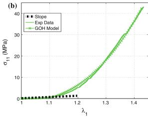
FIGURE 9. Nonlinear curve fitting to obtain the constitutive parameters:  $\mu$  and  $k_1$  are related to the early (infinitesimal) stress-strain part of the graph, see (a);  $k_2$ , to the rest of the curve.
