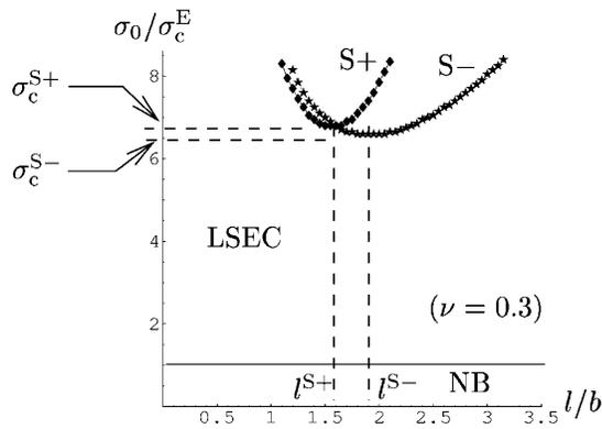
FIG. 2. Diagram of linear stability of the Euler column: no buckling (NB), linearly stable Euler column (LSEC), unstable Euler column by secondary antisymmetric buckling ( $S^-$ ), or secondary symmetric buckling ( $S^+$ ).
