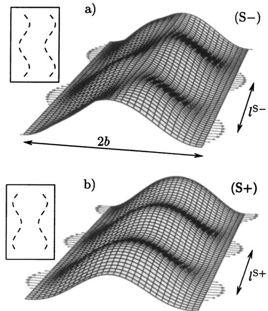
FIG. 4. Secondary buckling of the Euler column under the effect of the residual longitudinal compression (amplitude of the deflection is arbitrary). When (a)  $\nu = 0.3$  the most unstable mode is antisymmetric ( $S^-$ ), while (b) for  $\nu = 0.2$ , it is symmetric ( $S^+$ ). Instability of the delamination front caused by this secondary buckling has been represented by the lateral arrows, leading to delamination patterns in the insets.
