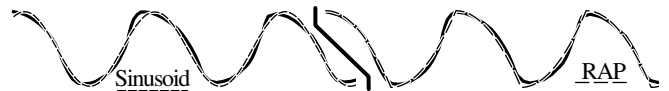
FIG. 1: The experimental crack path used in Ref. [1] (solid curve) is much better fitted by our two reference models than by the cycloidal construction (compare to their Fig. 2c).
