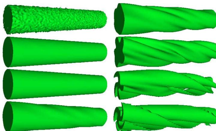
Figure 2: Time evolution of a initially stable Batchelor vortex when submitted to time varying strain at  $Re = 670$  (half-period of axial compression followed by half-period of axial stretching).
