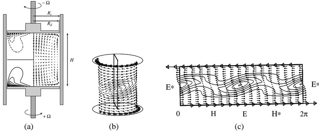
Figure 3: (a) Experimental configuration. The inset illustrates azimuthal velocity contours (left) and meridional velocity field (right) of the axisymmetric flow determined by numerical simulation [30]. (b) Velocity field and radial vorticity at a fixed radius showing a steady corotating pair of vortices. (c) Unrolled quantities as in (b).
