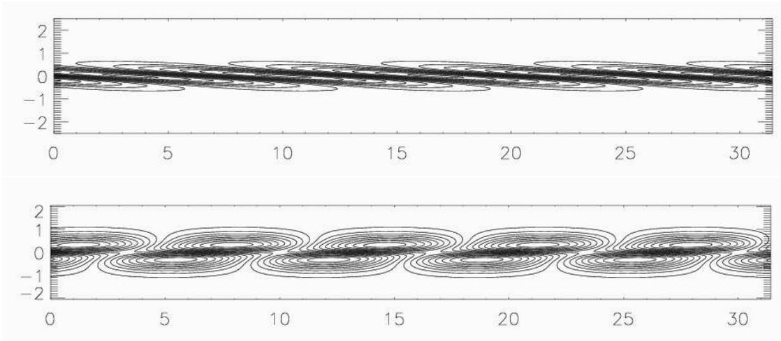
Figure 4: Vorticity isocontours of the most amplified perturbation at  $t = 20$  for a stretched shear layer. Top: at  $t = 0$ ; bottom: at  $t = 20$ .
