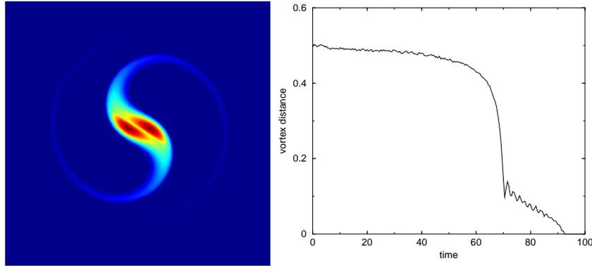
Figure 1: left: Vorticity field during merging for  $Re = 15.000$  at time  $t = 70$ ; right: vortex distance with respect to time.
