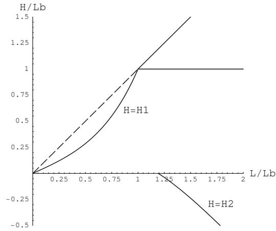
Figure 9: Extended version of fig.7 with the new curve  $H = H_2(L/L_b)$  where diving states lose stability as the end of the beam detaches from the interface.
