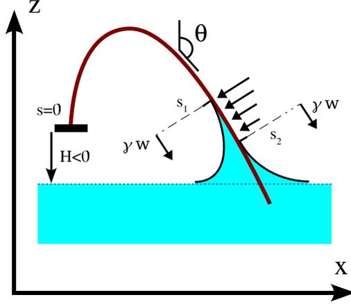
Figure 22: A diving beam, piercing the surface once.
