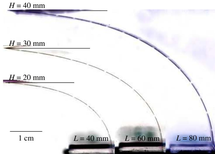
Figure 20: For the same ratio  $H/L$ , lightly deflected shapes are homothetic.
