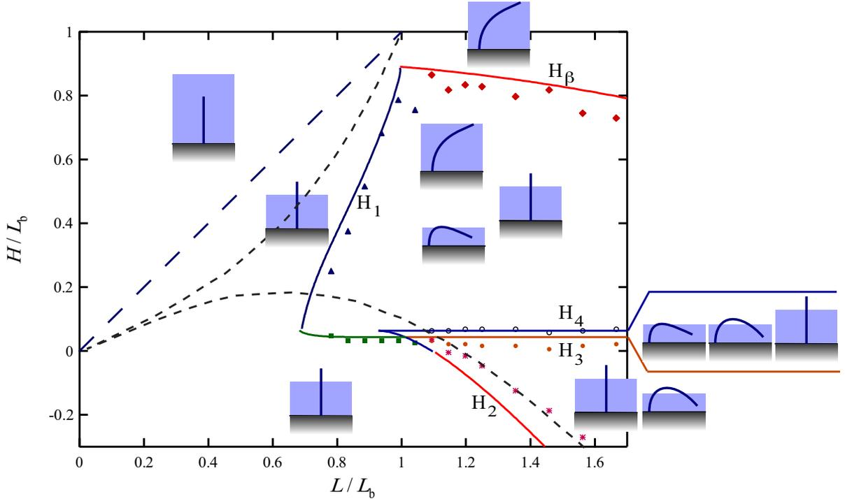
Figure 17: Experimental (symbols) and numerical (continuous lines) phase diagram for the elastic strip of thickness  $e = 25\mu\text{m}$  ( $L_b = 1.9\text{ cm}$ ). In each region of the diagram the different stable configurations are sketched. The numerical computations include gravity and finite meniscus sizes, whereas dashed curves (corresponding to curves  $H_1$  and  $H_2$ ) obtained without gravity at zero capillary length ( $L_c = 0$ ) are drawn as guides to the eye.
