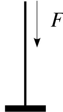
max. capillary force (on straight beam)  $F_{tot} = 2 \gamma w$
