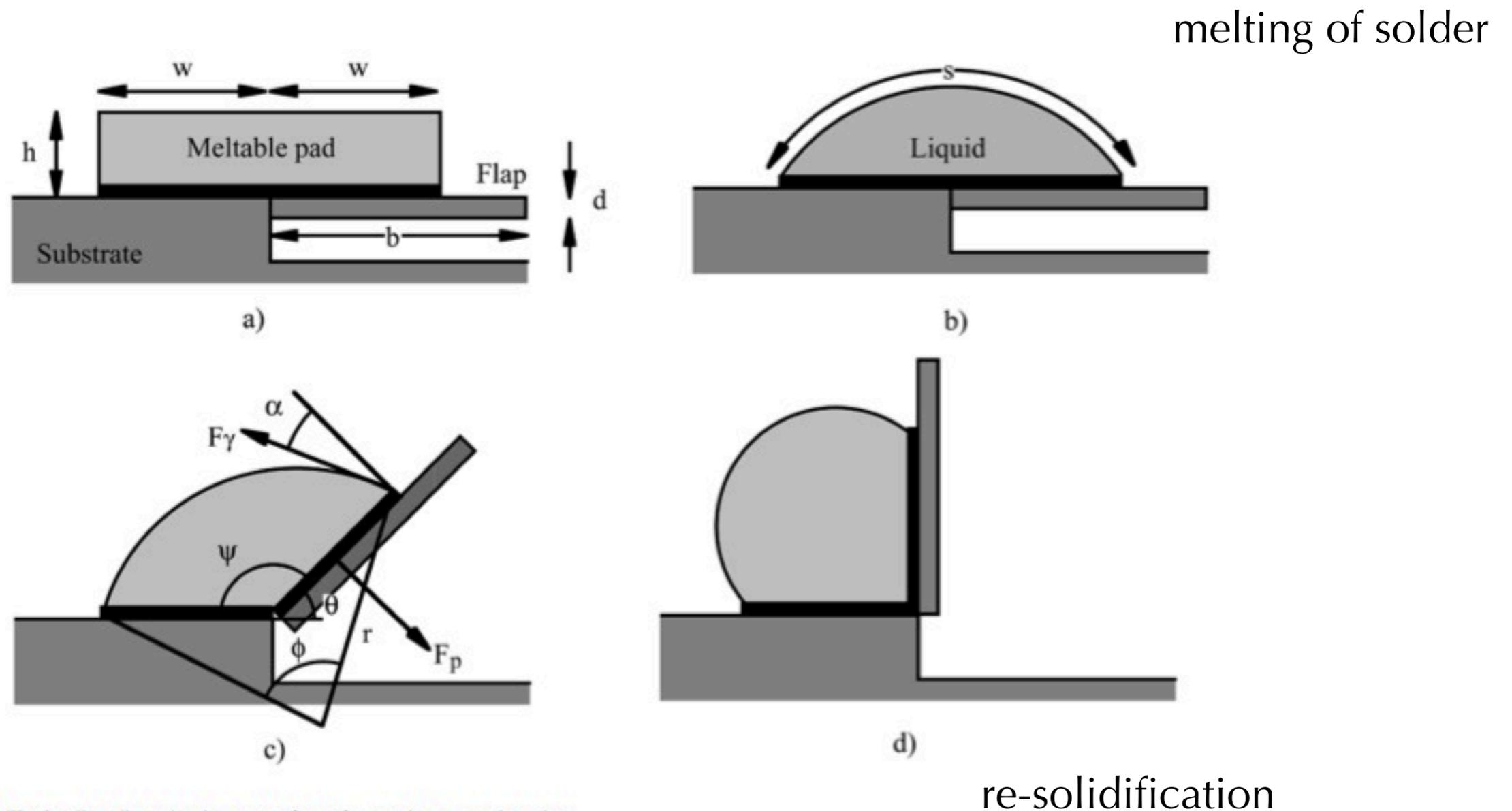
Fig. 3. Two-dimensional geometry for surface tension powered rotation.
