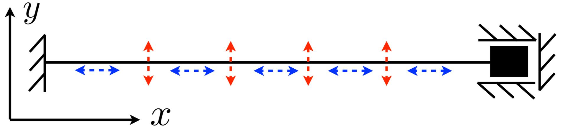
flexural vib.  $y'''' + \bar{p}y'' - \bar{\omega}^2 y = 0$  with  $\begin{cases} \bar{p} = p(1 - \epsilon p) \\ \bar{\omega} = \omega(1 - \epsilon p) \end{cases}$
