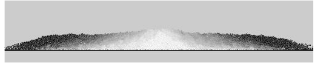
Figure 1. Snapshot of the spreading process. The gray shade shows the velocity of the grains. White corresponds to zero velocity, while black indicates the maximum velocity.
