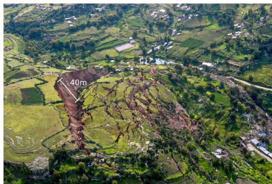
Figure 1: Picture of a landslide which occurred in Llusco (Peru), in 2018. This collapse is typical of a cohesive granular flow, featuring a first fracture plane, with secondary fractures transverse to the flow.
