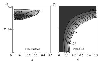
FIGURE 5. Influence of the free surface on the bar instability in a purely viscous flow (Re = 0 and S = 0.02 for both plots). (a) The flow has a free surface, with vanishing surface tension ( $Bo \to \infty$ ). (b) The flow is covered with a rigid lid. In figure (b) the colour scale has been modified in order to show negative contours. The values of the other flow parameters are the same as in figure 3.
