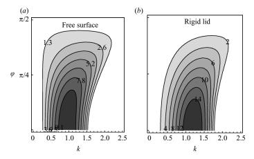
FIGURE 4. Influence of the free surface on the ripple instability (Re = 27 and S = 0.01 for both plots). (a) The flow has a free surface, with vanishing surface tension ( $Bo \to \infty$ ). (b) The flow is covered with a rigid lid, at  $\tilde{z} = 2$ , so that the base-flow profile is the complete Poiseuille parabola, which lower half corresponds exactly to the Nusselt film of the free-surface case. The values of the other flow parameters are the same as in figure 3.
