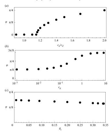
FIGURE 8. Sensibility of the bar instability mode with respect to the parameters of the sediment transport law. The black disks indicate the angle  $\varphi$  of the maximum. The flow parameters correspond to a real case, for which F = 0.51, S = 0.02, Bo = 0.5, Sh = 0.34 and  $\mathcal{U}d_s^2/(U_s\mathcal{D}^2) = 0.08$ . The transport law parameters are set to  $\theta_t = 0.091$ ,  $c_u/c_d = 1.5$  and  $c_g = 0.11$ , except naturally for the one involved in each plot.
