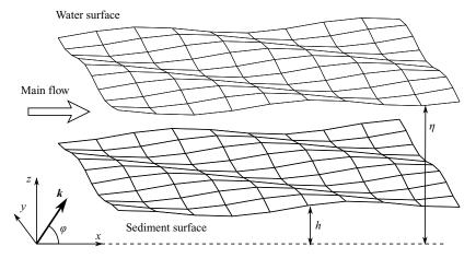
FIGURE 2. Schematic of the system and associated notations. A film of fluid with a free surface flows over a granular layer. In  $\S 3$ , the stability of a perturbation with wave vector k is analysed.
