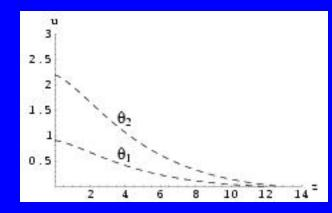
Continuum mechanical model for dense sheared flow which accounts dilatance effect and amounts for both volume fraction and velocity field
