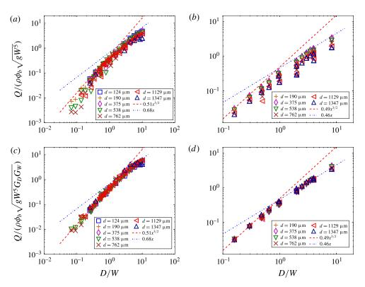
FIGURE 13. (Colour online) Mass flow rate Q as a function of D/W for various d for (a,c) rectangular silos and (b,d) cylindrical silos, normalised in (a,b) by  $(\rho\phi_b\sqrt{gW^5})$  and in (c,d) by  $\rho\phi_b\sqrt{gW^5}G_D(D/d)G_W(W/d)$  (see (3.12)) with the fitting parameters  $\beta_D=\beta_W=0.1$ ,  $\alpha_D=1$  and  $\alpha_W=0.46$  (see appendix A). The dashed and dashed-dotted lines are the same as in figures 5 and 12.
