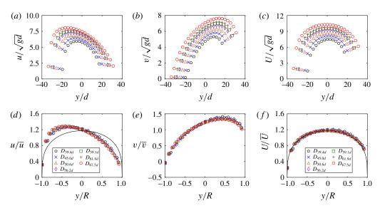
FIGURE 18. (Colour online) Two-dimensional continuum simulation (a,d) horizontal velocity (b,e) vertical velocity and (c,f) norm of the velocity, (a-c) normalised by  $\sqrt{gd}$  versus y/d and (d-f) normalised by the mean value versus y/R, the full lines in (d,f) represent equation (A 5) with  $v_v = 0.31$ .
