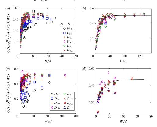
FIGURE 14. (Colour online) Experimental results obtained with rectangular silos: dimensionless flow rate  $Q/(\rho\phi_bWDF(D/W)\sqrt{gD})$  versus (a,b) D/d and (c,d) W/d. Selected experimental runs: (a,c) all the runs, (b) D<1.8W and W>10d, (d) D>2.2W and D>20d. The full lines represent the geometrical functions  $G_D(D/d)=[1-\alpha_D e^{-\beta_D(D/d)}]$  and  $G_W(W/d)=[1-\alpha_W e^{-\beta_W(W/d)}]$  with  $\alpha_D=1$ ,  $\beta_D=0.1$ ,  $\alpha_W=0.46$  and  $\beta_W=0.1$  respectively.
