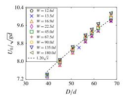
FIGURE 10. (Colour online) Continuum simulation results: norm of the velocity  $U_0/\sqrt{gd}$  on the central streamline at the orifice versus D/d for various W. The dashed line represents equation (3.9) with  $c_U = 1.2$ .
