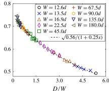
FIGURE 9. (Colour online) Continuum simulation results: angle of inclination  $\theta$  of the central streamline at the orifice relative to vertical for various W (a) versus D/U, (b) versus D/W. The dashed line represents equation (3.11) with  $\gamma_1 = 0.56$  and  $\gamma_2 = 0.25$ .
