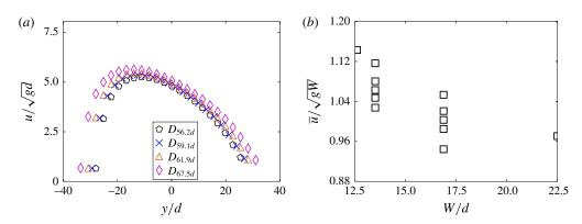
FIGURE 20. (Colour online) Pseudo-3-D continuum simulation. (a) Horizontal velocity normalised by  $\sqrt{gd}$  versus y/d at the outlet for different D and W=13.5d; (b) mean horizontal velocity normalised by  $\sqrt{gW}$  for D/W>3.
