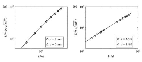
FIGURE 17. Flow rate made dimensionless by  $\sqrt{gd^3}$  versus the number of beads in the aperture D/d for the 2-D case, (a) discrete simulation, (b) continuum simulation. The full lines represent equation (A 9) with (a)  $C'_l = 1.08$  and (b)  $C'_l = 0.78$ .
