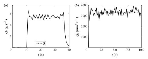
FIGURE 2. Temporal evolution of the instantaneous flow rate. (a) Experiment with rectangular silo,  $d = 190 \mu m$ , D = 10 mm and W = 3.5 mm. (b) Two-dimensional discrete simulation with d = 2 mm and D = 16 mm. The dashed lines represent the mean flow rate Q.
