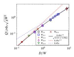
FIGURE 12. (Colour online) Experimental results in the cylindrical silo: dimensionless mass flow rate  $Q/(\rho\phi_b\sqrt{gW^5})$  as a function of the aperture aspect ratio D/W. The dashed line represents equation (3.2) with  $c_D=0.49$ , and the dashed-dotted line represents equation (3.3) with  $c_W=0.46$ .
