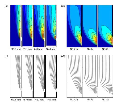
FIGURE 7. (Colour online) Velocity field (a,b) and streamlines (c,d) for the experiment (a,c) with D=20 mm, d=1129  $\mu$ m and W=[3.5, 10, 20, 40] mm, and for the continuum simulation (b,d) with D=56.25d and W=[13.5d, 45d, 180d].
