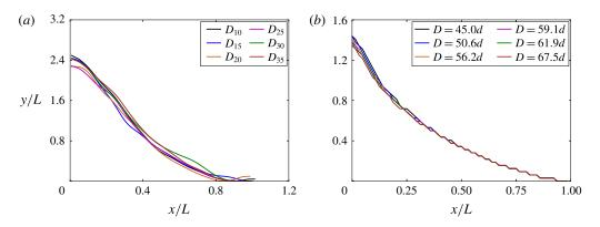
FIGURE 8. (Colour online) Limit of the stagnant zone for various D: (a) experiments with W = 5 mm and (b) continuum simulations with W = 17.4d.
