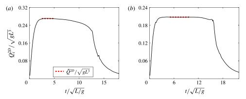
FIGURE 3. (Colour online) Continuum simulation: temporal evolution of the dimensionless instantaneous flow rate  $Q_i^{2D}/(\sqrt{gL^3})$ , as a function of the dimensionless time  $t/\sqrt{L/g}$  for L=90d and D=0.5L (a) in two dimensions (b) in pseudo three dimensions with W=22.5d. The dashed lines represent the mean flow rate  $Q^{2D}/(\sqrt{gL^3})$ .
