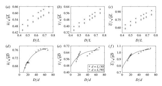
FIGURE 19. Two-dimensional continuum simulation: (a,d) horizontal velocity, (b,e) vertical velocity and (c,f) norm of the velocity normalised in (a-c) by  $\sqrt{gL}$  versus D/L and normalised in (d-f) by  $\sqrt{gD}$  versus D/d for two particles diameters. The full lines in (d-f) represent equation (A 7) with the fitting parameters  $\beta=0.05$ ,  $\xi_u=0.78$ ,  $\alpha_u=0.25$ ,  $\xi_v=0.68$ ,  $\alpha_v=0.31$ ,  $\xi_U=1.06$  and  $\alpha_U=0.28$  obtained using the least-squares method.
