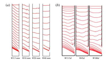
FIGURE 11. (Colour online) Profiles of the top surface of granular materials for various W at constant time steps: (a) experiments with D=25 mm, d=190  $\mu$ m, time interval  $\Delta t_e=0.5$  s, (b) continuum simulation with D=56.25d and time interval  $\Delta t_s/\sqrt{d/g}=9.5$ .
