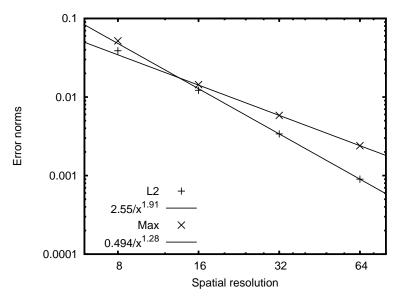
FIGURE 3. Convergence of the error norms of the difference between the computed velocity and the exact Bagnold solution error norms  $L^2$  and max as a function of resolution (number of grid points across the granular layer).
