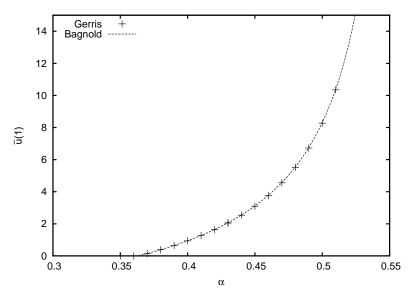
FIGURE 4. In the case of a single granular layer  $(0 < \bar{y} < 1)$ , comparison between numerical (+) and analytical (dashed line) solutions for the velocity at the surface  $\bar{u}(\bar{y}=1)$  as a function of the slope angle  $\alpha$ . For  $\alpha < \arctan(\mu_s) \simeq 0.363$  there is no motion, as expected.
