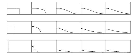
FIGURE 7. Strip representing a series of snapshots of a column collapse with aspect ratio a=0.5, 1.42, 6.26 (from top to bottom) simulated with Gerris at time  $\bar{t}=0, 1, 2, 3, 4$ . The surrounding fluid is Newtonian of density  $\rho_f$  and viscosity  $\eta_f$ , while the non-Newtonian  $\mu(I)$ -rheology is used for the column.
