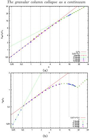
FIGURE 12. (a) Normalised run-out  $(L_{\infty} - L_0)/L_0$  and (b) normalised final height  $H_{\infty}/L_0$  as functions of the aspect ratio a for  $\mu(I)$  continuum simulations. The different sets of symbols correspond to increasing spatial resolutions.
