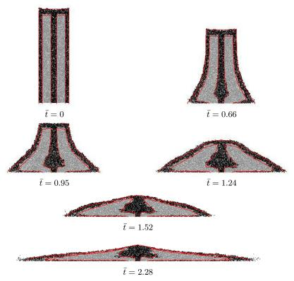
FIGURE 10. Comparison between the  $\mu(I)$  continuum model (red line) and contact dynamics simulations (grains) for an aspect ratio a=6.26 at different times (non-dimensionalized by  $\sqrt{H_0/g}$ ). The parameters of the  $\mu(I)$ -rheology are  $\mu_s=0.32, \ \Delta\mu=0.28$  and  $I_0=0.4$  (color online).
