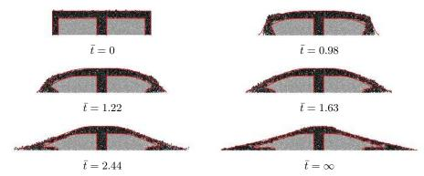
FIGURE 8. Comparison between the  $\mu(I)$  continuum model (red line) and contact dynamics simulations (grains) for an aspect ratio a=0.5 at different times (non-dimensionalized by  $\sqrt{H_0/g}$ ). The grains are colored in the initial heap, which allows one to track the displacement, see (Staron & Hinch 2005). The parameters of the  $\mu(I)$ -rheology are  $\mu_s=0.32, \ \Delta\mu=0.28$  and  $I_0=0.4$ . (color online).
