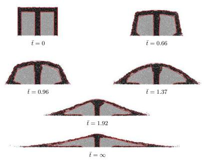
FIGURE 9. Comparison between the  $\mu(I)$  continuum model (red line) and contact dynamics simulations (grains) for an aspect ratio a=1.42 at different times (non-dimensionalized by  $\sqrt{H_0/g}$ ). The parameters of the  $\mu(I)$ -rheology are  $\mu_s=0.32,~\Delta\mu=0.28$  and  $I_0=0.4$  (color online).
