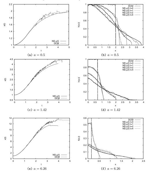
FIGURE 11. Normalised position of the flow front  $x/L_0$  as a function of the normalised time  $\bar{t}=t/(H_0/g)^{1/2}$  and height profiles at different instants  $t\sqrt{g/H_0}=0$ , 1, 2, and 4, in the case of columns of aspect ratios a=0.5 ((a) and (b) respectively), a=1.42 ((c) and (d) respectively) and a=6.26 ((e) and (f) respectively), for discrete contact dynamics simulation (noisy dashed line) and continuum Gerris simulation with the  $\mu(I)$ -rheology (plain line).
