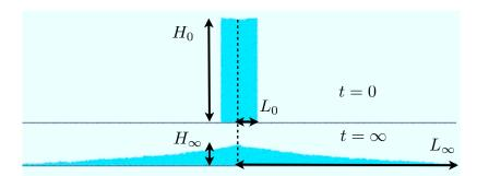
FIGURE 6. Schematic illustration of the column collapse experiment in two dimensions. The initial height of the column is  $H_0$ , its initial half-width is  $L_0$  and  $a = H_0/L_0$  is the aspect ratio; the final maximum thickness is  $H_{\infty}$  and the final half-width, or run-out, is  $L_{\infty}$ .
