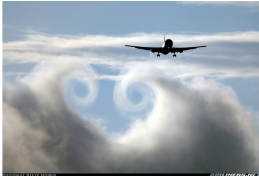
FIGURE 12 – Two trailing wing vortices. Steve Morris http://www.airliners.net
