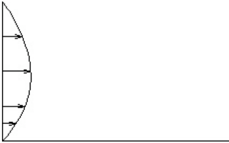
Figure 8: Basic Poiseuille profile, [click on the Image, Acrobat QuickTime Required] to see the effect of aspiration
