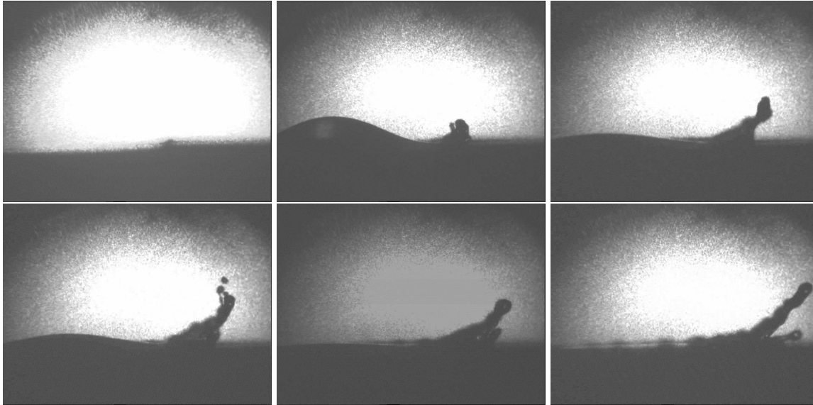
FIGURE 1. Impact on the 0.035mm obstacle (from left to right and top to bottom : void, 1000ms, 1250ms, 1500ms, 2000 ms and 2500 ms)
