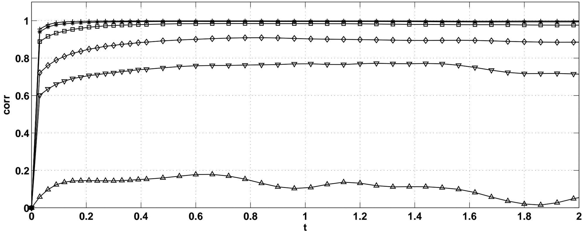
Estimation transient for the streamwise velocity  $u$  at  $y^+ = 1.5$ ,  $y^+ = 5.5$ ,  $y^+ = 9.7$ ,  $y^+ = 19.8$ ,  $y^+ = 31.5$ , and along the channel centreline
