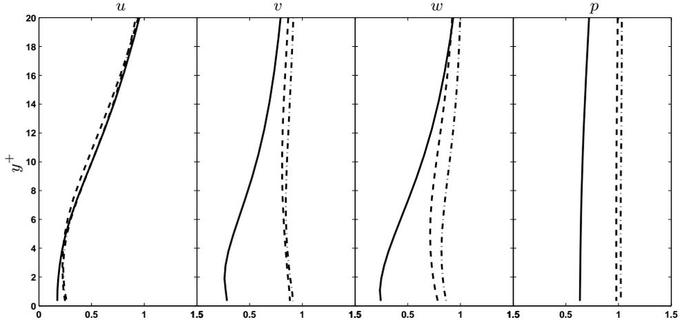
FIGURE 7. The relative estimation error  $\text{err}_{\eta_y}(s, \hat{s})$ , defined as in equation (5.2) plotted for the Kalman filter. The solid line denotes estimation performed with all three measurements and gains based on turbulence statistics. The dashed line denotes the estimator performance using only the  $\eta_y$  measurement. The dash-dotted line is the correlation when using the spatially uncorrelated stochastic model.
