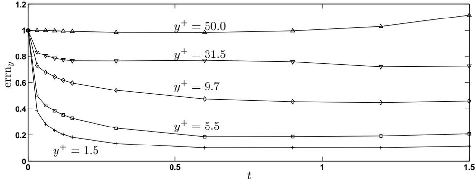
FIGURE 10. The transient behavior of the total error energy at  $y^+ = 1.5$ ,  $y^+ = 5.5$ ,  $y^+ = 9.7$ ,  $y^+ = 31.5$ , and along the channel centerline for case 3 in table 1. All three measurements are used together with the Kalman filter.
