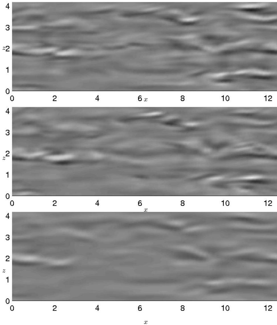
FIGURE 11. Wall-normal velocity component  $v$  plotted at  $y^+ = 9.7$  at an instant in time. In the top figure the flow velocity itself is plotted. The middle plot shows the velocity field reproduced by the extended Kalman filter, and the bottom plot shows the velocity field reproduced by the Kalman filter. The contour levels range from  $-1$  to  $1$ , where black and white represent the lower and upper bound respectively.
