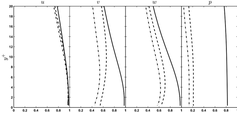
FIGURE 5. The figure shows  $\text{corr}_y(s, \hat{s})$  for  $s = u$ ,  $s = v$ ,  $s = w$ , and  $p$  obtained using Kalman filter. The solid line denotes estimation using all three measurements and noise statistics as discussed in §3. The dashed line denotes the estimator performance using only the  $\eta_y$  measurement. The dash-dotted line is obtained using the spatially uncorrelated stochastic model for noise statistics.
