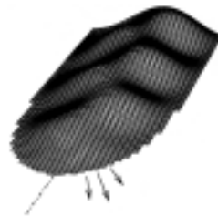
FIG. 5. A mechanism of instability leading to undulations in a finger of delamination: longitudinal buckling in the tail of the blister breaks the symmetry at the tip, and favors oblique propagation.
